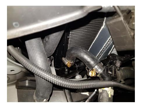
INSTALL TOP HOSE WITH SHORT SIDE TO HEAT EXCHANGER USING HOSE CLAMPS SUPPLIED. OPEN DRAIN VALVE ON THE REAR OF THE HEAT EXCHANGER AND ADD COOLANT TO THE COOLANT RESERVIOR UNTIL COOLANT COMES OUT OF THE BLEED VALVE. (APPROX 2 LITRES). TIGHTEN BLEED VALVE. LET SIT FOR APPROX 15 MIN AND RE CHECK LEVELS. REMOVE CLAMPS.
