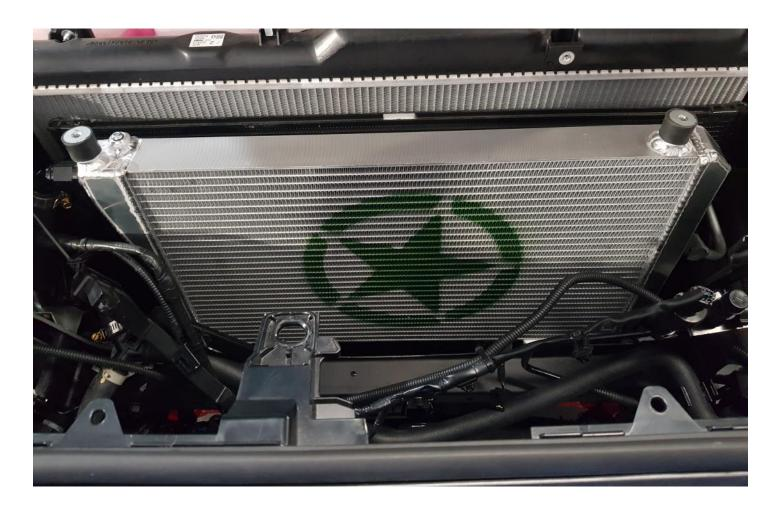
INSTALL LOWER HOSE WITH LONG END TO HEAT EXCHANGER WITH HOSE CLAMPS SUPPLIED.
