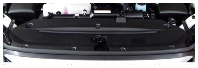
REMOVE PLASTIC COVER OVER BONNET LATCH. MARK POSITION AND UN BOLT BONNET LATCH ALONG WITH SUPPORT BRACKET. UN PLUG HORNS AND UNPICK THE WIRING LOOM RUNNING UNDER THE RADIATOR SUPPORT PANEL. UN BOLT AC PIPE SUPPORT BRACKET AND REMOVE CENTRE RADIATOR SUPPORT PANEL. REMOVE PLASTIC SUPPORT FROM THE BONNET LATCH CABLE AND INSTALL SUPPLIED CONDUIT.
