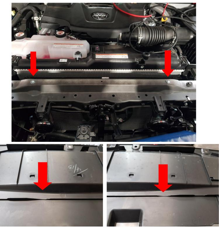
ON THE UNDER SIDE OF THE PLASTIC COVER REMOVE MATERIAL LIKE SHOWN TO CLEAR THE ALLEN HEAD BOLTS.
