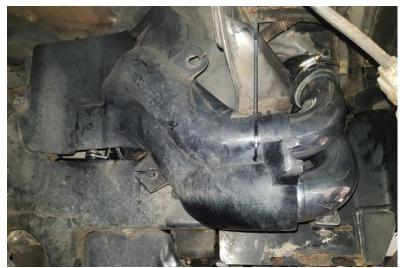
INSTALL 8MM P CLAMP TO AC MOUNTING BOLT.
