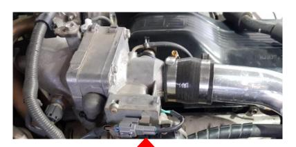
INSTALL SUPPLIED 3MM VACUUM HOSE FROM OIL SCAVANGE FITTING ON THE INTERCOOLER TO THE FITTING ON THE CROSSOVER PIPE AS SHOWN. SECURE WITH CABLE TIES.
