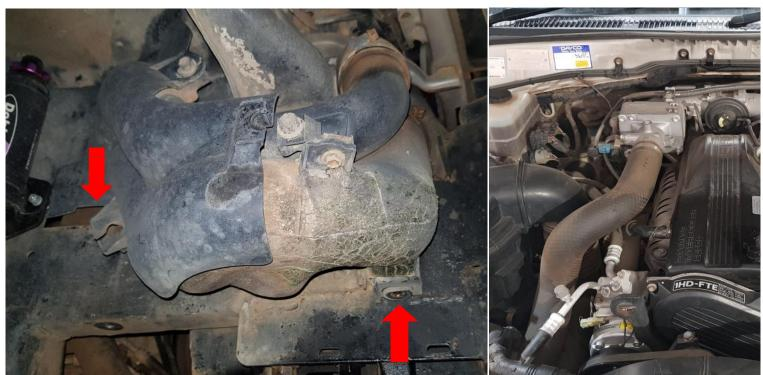
REMOVE APPROX 3-4MM OF MATERIAL LIKE SHOWN FROM THE RADIATOR SUPPORT PANEL. THIS IS TO ALLOW CLEARENCE FOR THE INTERCOOLER. THE DRIVERS SIDE LOWER CONDENSOR BRACKET WILL ALSO NEED TO BE TRIMMED AS SHOWN, REMOVE THE LIP OFF THE TOP OF THE BOLT HOLDING THE CONDENSOR BRACKET.
