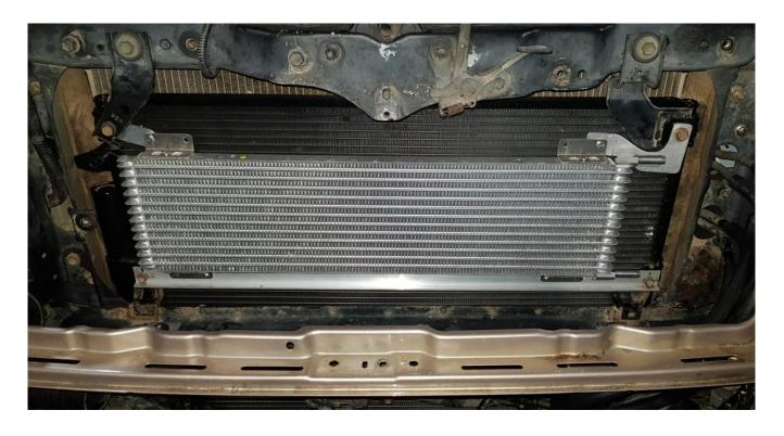
INSTALL THE TWO LONG TRANS COOLER HOSES LIKE SHOWN USING HOSE CLAMPS SUPPLIED.
