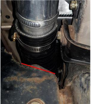
DEPENDING WHAT BULL BAR IS FITTED, REMOVE MATERIAL SHOWN FOR ADDED CLEARENCE.
