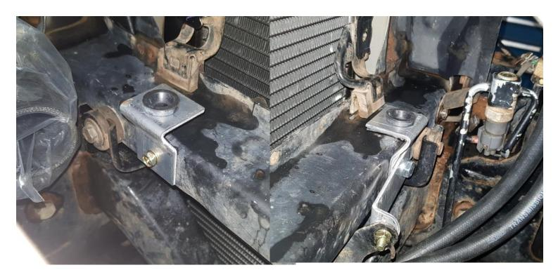
INSTALL THE TRANSCOOLER TO THE LOWER BRACKET SUPPLIED USING THE M5 BOLTS AND NUTS AND TIGHTEN. INSTALL THE TOP BRACKETS AS SHOWN LEAVING LOOSE. INSTALL THE TRANS COOLER WITH BRACKETS ATTACHED TO THE CONDENSOR SUPPORT BRACKETS AS SHOWN HAVING THE DRIVERS SIDE BETWEEN THE BRACKET AND CONDENSOR AND THE PASSANGER SIDE INFRONT OF THE BRACKET LIKE SHOWN. TIGHTEN ALL BOLTS.
