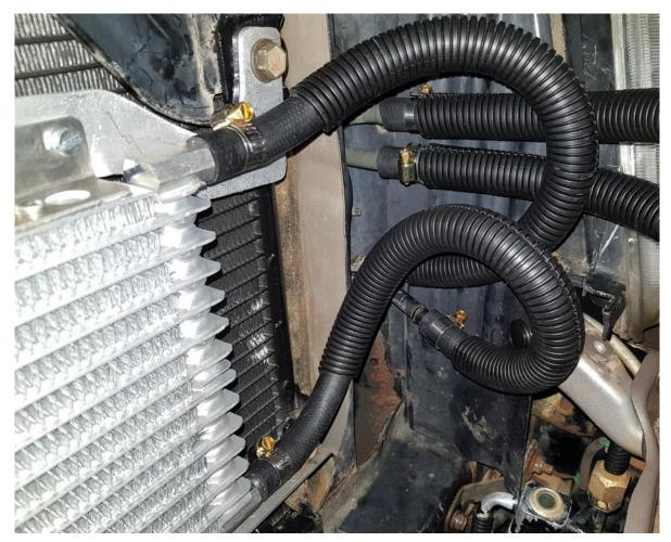
CAREFULLY INSTALL THE INTERCOOLER BY ORIENTATING THE INTERCOOLER HORIZONTALY PUTTING THE DRIVERS SIDE IN PARTIALLY FOLLOWED BY THE PASSANGER SIDE BEING CAREFUL NO TO DAMAGE THE TRANS COOLER. WITH THE INTERCOOLER IN PLACE INSTALL THE TOP SUPPORT BRACKETS WITH SUPPLIED M8X25 BOLTS.
