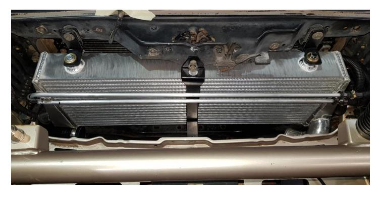
INSTALL THE OIL SCAVANGE FITTING TO THE BOTTOM OF THE INTERCOOLER. INSTALL THE RADIATOR SUPPORT BRACKET USING THE FACTORY NUT AND BOLT TOP AND BOTTOM AND THE M6X16 ALLEN HEAD IN POSITION SHOWN. AFTER THE CENTRE BRACKET IS IN PLACE INSTALL THE POWER STEERING COOLER TUBE IF APPLICABLE USING THE 3 SMALL P CLAMPS AND M6X12 ALLEN HEAD BOLTS. CONNECT POWER STEERING COOLER TO HOSES PREVIOUSLY FITTED USING HOSE CLAMPS SUPPLIED.
