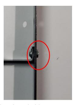
REINSTALL THE HORNS AND BRACKET AND BONNET LATCH, REINSTALL GRILL USING SUPPLIED UPPER GRILL SUPPORT WITH M5 HEX BOLT AND NUT.
