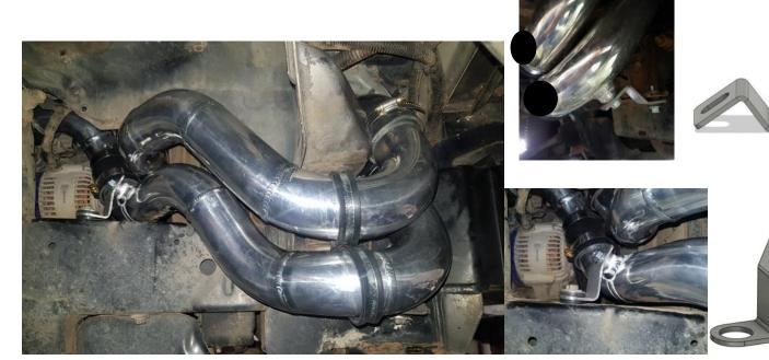
IF AN AFTERMARKET TURBO IS INSTALLED TRIM THE DIFF BREATHER BRACKET AS SHOWN AND USE P CLAMP TO MOUNT EARTH CABLE. INSTALL P CLAMP TO THE BOTTOM AC BOLT MOUNTING BOLT AS SHOWN AND CABLE Tie ALTERNATOR CABLE AWAY FROM TURBO PIPE. USE THE 180 ALUMINIUM PIPE (SILICONE 180 SHOWN) AND SECOND ALUMINIUM PIPE SHOWN. WITH THE ADDITIONAL 90 DEGREE SILICONE. AND CONNECT BOTTOM PIEPWORK TO TURBO OUTLET.
