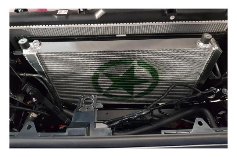
INSTALL LOWER HOSE WITH SHORT END TO HEAT EXCHANGER WITH HOSE CLAMPS SUPPLIED.
