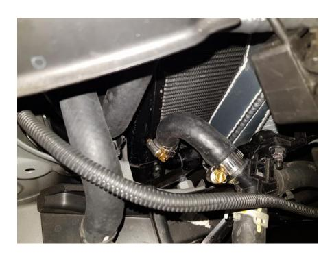
INSTALL TOP HOSE WITH SHORT SIDE TO HEAT EXCHANGER USING HOSE CLAMPS SUPPLIED.
