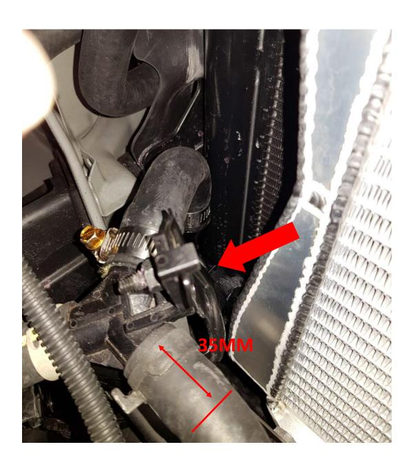
INSTALL THE LOWER MOUNTING BRACKETS TO THE LOWER CROSSBAR LIKE SHOWN USING THE M8X16 BOLT AND NUT. LEAVE FINGER TIGHT.
