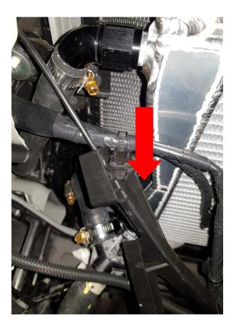
REINSTALL TOP RADIATOR SUPPORT PANEL ALONG WITH THE SUPPLIED M6X7 ALLEN HEAD BOLTS TO THE TOP RUBBER MOUNTS FOR THE HEAT EXCHANGER.
