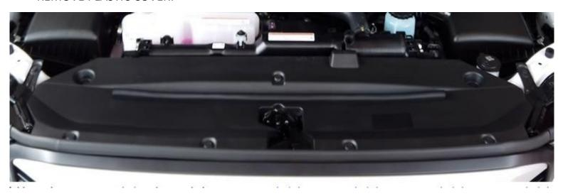
REMOVE PLASTIC COVER OVER BONNET LATCH. MARK POSITION AND UN BOLT ALONG WITH SUPPORT BRACKET. UN PLUG FANS AND UNPICK THE WIRING LOOM RUNNING UNDER THE RADIATOR SUPPORT PANEL. UN BOLT AC PIPE SUPPORT BRACKET AND REMOVE CENTRE RADIATOR SUPPORT PANEL.
