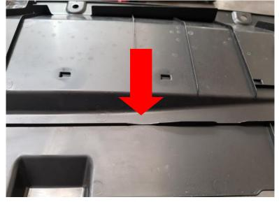
ON THE UNDER SIDE OF THE PLASTIC COVER REMOVE MATERIAL LIKE SHOWN TO CLEAR THE ALLEN HEAD BOLTS.
