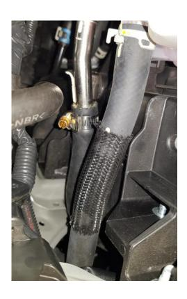
REMOVE THE PLASTIC BONNET RELEASE GUIDE AND SLIDE OVER CONDUIT SUPPLIED.
