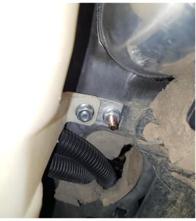
LOOSEN SCREW ON THE HEADLIGHT SUPPORT BRACKET AND PUSH TO THE CENTRE OF THE VEHICLE. TIGHTEN. CUT LIKE SHOWN. PAINT BARE METAL, LOOSEN SCREW AND PUSH BACK. RE TIGHTEN SCREW.
