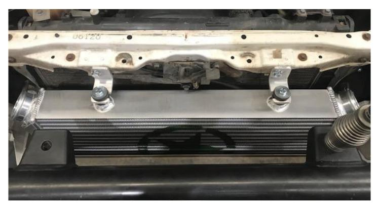
INSTALL THE MANIFOLD PIPE FIRST. THE INTERCOOLER MAY NEED TO BE LEANT FORWARD TO HELP INSTALL.
