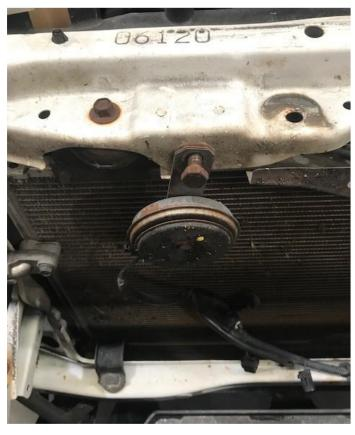
INSTALL SMALL BONNET LATCH SUPPORT BRACKET TO THE BONNET LATCH MECHANISM USING THE M6X10 HEX HEAD AND M8 WASHER.
