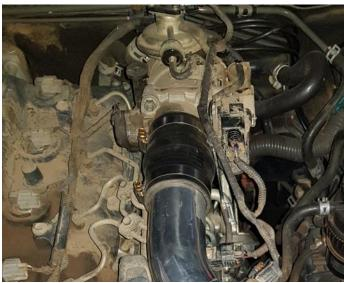
INSTALL THE INTERCOOLER TO THE LOWER MOUNTS USING THE SUPPLIED M8X35 BOLTS.
