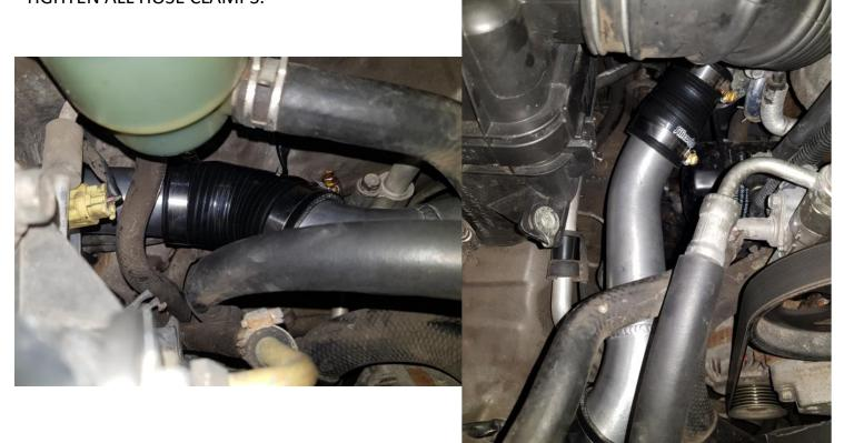
INSTALL 2 1/4" 90 DEGREE SILICONE (SHORT SIDE) TO THE INTERCOOLER FOLLOWED BY THE MANIFOLD SIDE PIPE WITH THE SUPPORT BRACKETS. BOLT BRACKET IN PLACE WITH THE M8X35 BOLTS SUPPLIED THROUGH THE FACTORY RUBBERS.
