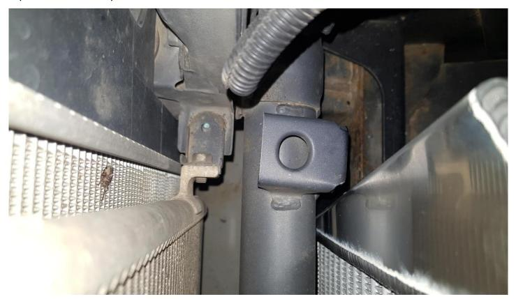
**Step 4** Lower the intercooler into position from the top and be sure the coolers locating dowels insert into the lower mounts rubbers. Using the supplied M8x25 safety bolt, fasten top cooler mount and horn to the bonnet latch support. Your upgraded cooler is now bolted firmly in place.
