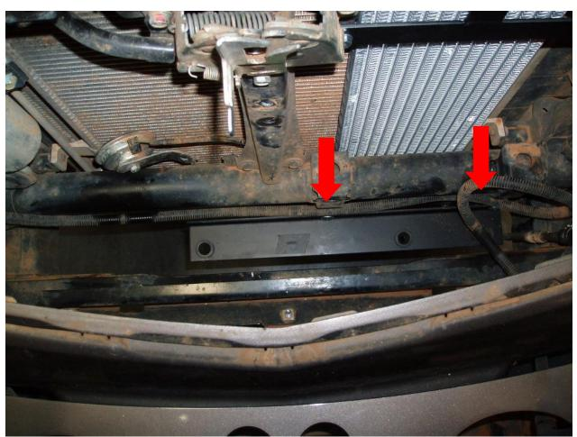
WHEN INSTALLING THE INTERCOOLER CHECK THERE IS CLEARENCE TO THIS BRACKET (PASSENGER SIDE).
