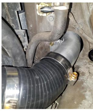
INSTALL THE REDUCER, 2: ALUMINIUM PIPE AND 2: 45 DEGREE (LONG SIDE TO TURBO) AS SHOWN.
