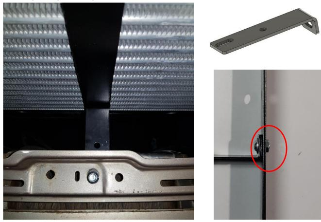
REINSTALL THE HORNS AND BRACKET AND BONNET LATCH, REINSTALL GRILL USING SUPPLIED UPPER GRILL SUPPORT WITH M5 HEX BOLT AND NUT.
