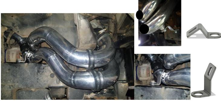
IF AFTER MARKET TURBO, INSTALL PIPE 5 IN PLACE OF PIPE 4, AND 2"-2 1/4" 135 DEGREE REDUCER IN PLACE OF THE STRAIGHT REDUCER. SOME TRIMMING OF THE SILICONE MAY BE REQUIRED.
