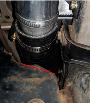
DEPENDING WHAT BULL BAR IS FITTED, REMOVE MATERIAL SHOWN FOR ADDED CLEARENCE. INSTALL THE LOWER INTERCOOLER BRACKETS. WITH THE 6MM SLOTED BRACKET TO THE DRIVERS SIDE AND THE 8MM SLOTED BRACKET TO THE PASSANGER SIDE. INSTALL BOLT TO THE CENTRE OF THE SLOT.
