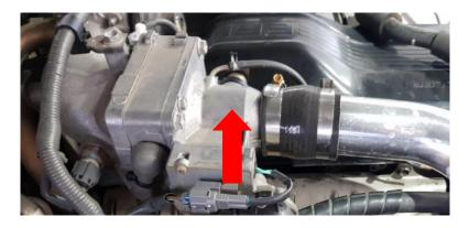
INSTALL SUPPLIED 3MM VACUUM HOSE FROM OIL SCAVANGE FITTING ON THE INTERCOOLER TO THE FITTING ON THE CROSSOVER PIPE AS SHOWN. SECURE WITH CABLE TIES. INSTALL THE LOWER GRILL SUPPORT BRACKET WITH THE M6X10 ALLEN HEAD BOLT AND M6 HALF NUT. CONFIRM THERE IS CLEARENCE BETWEEN THE HALF NUT AND INTERCOOLER. MOUNT TO SKIRT PANEL WITH M5 HEX BOLT AND NUT.
