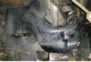
INSTALL 8MM P CLAMP TO AC MOUNTING BOLT. FIX LOWER SECTION OF PIPE TOGETHER USING P CLAMPS LIKE SHOWN .
