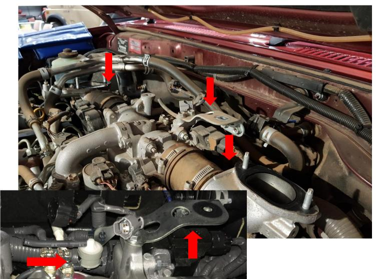
REMOVE STEEL HEATER LINES AND RUBBER HOSES GOING TO THE MOTOR. INCLUDING THE ONE SHOWN BELOW.
