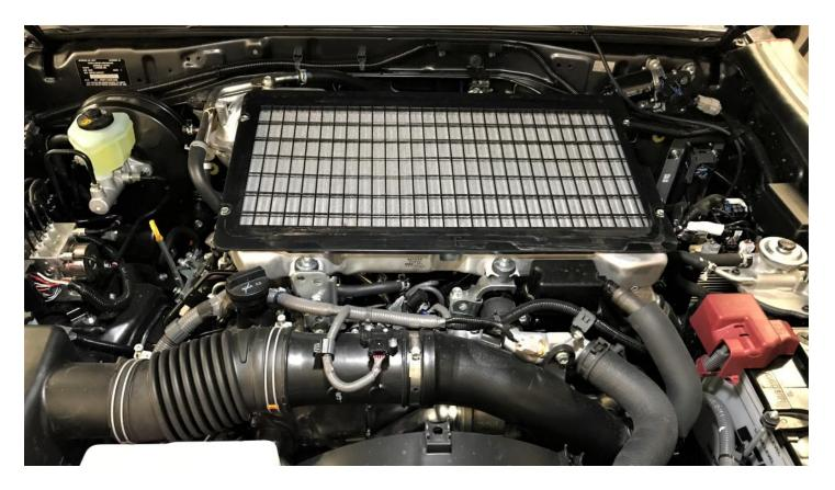
DISCONNECT MAP AND TEMP SENSOR (AT THE REAR OF THE INTERCOOLER). REMOVE FACTORY INTERCOOLER, PIPEWORK TO THE THROTTLE BODIES AND HOSE OFF THE TURBO PIPE. REMOVE MAP SENSOR FILTER OFF THE BRACKET SHOWN AND REMOVE BRACKET.
