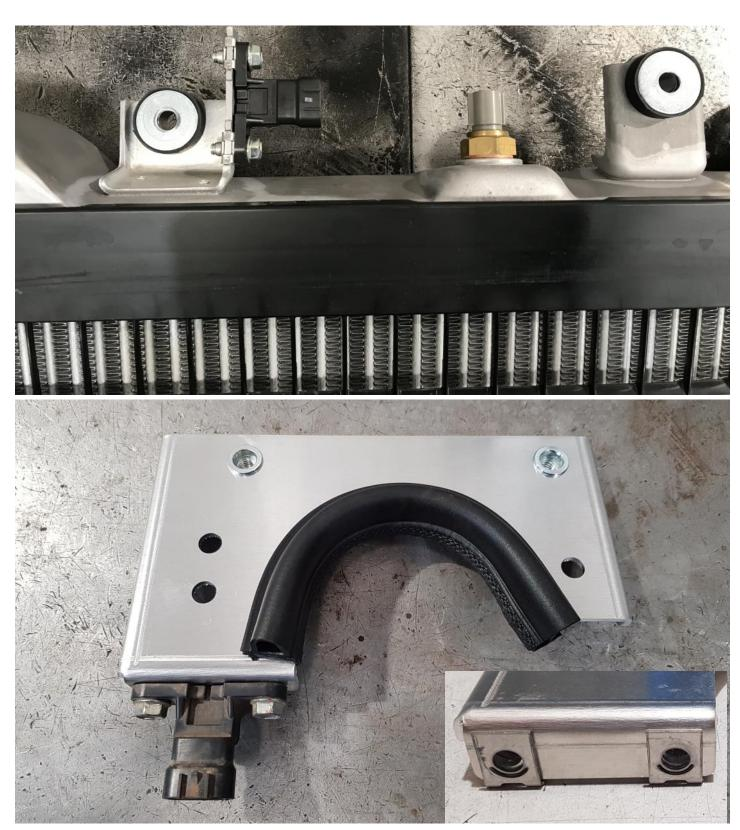
INSTALL THE REAR INTERCOOLER BRACKET AS SHOWN USING SUPPLIED M8X16 ALLEN HEAD BOTLS TO THE CENTRE OF THE SLOT. DUMMY FIT THE INTERCOOLER AND ADJUST IF NEEDED. CONNECT MAP SENSOR ELECTRICAL CONNECTOR AND MAP SENSOR VACUUM LINE.
