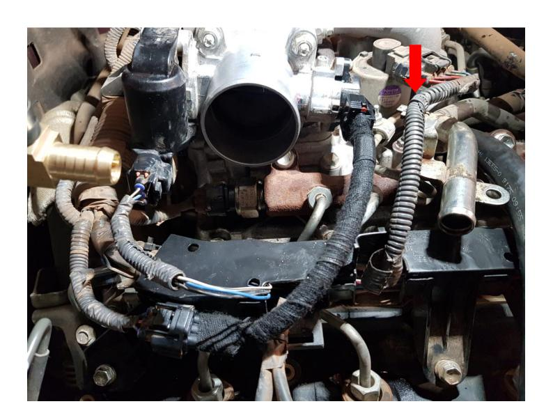
REMOVE THE MOUNTING RUBBERS AND WASHERS (FRONT AND REAR), TEMP SENSOR AND MAP SENSOR INCLUDING SPEED CLIPS FROM THE FACTORY INTERCOOLER. INSTALL THE TEMP SENSOR INTO INLET ADAPTOR USING FACTORY BRASS WASHER. INSTALL MOUNTING RUBBERS TO THE NEW INTERCOOLER FOLLOWED BY THE CRUSH TUBE WASHERS.
