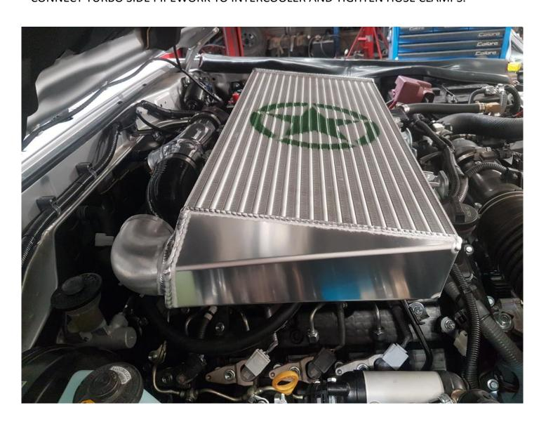
INSTALL REAR PIPEWORK AS SHOWN. DUE TO MINOR VARIATIONS BETWEEN VEHICLES THE 45 DEGREE SILICONE IS SUPPLIED LONG AND MAY NEED TO BE TRIMMED.
