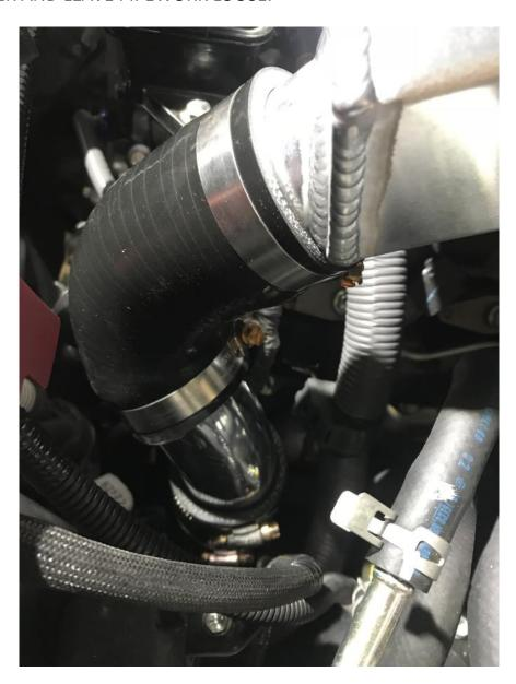
MAKE SURE THE FAN WIRES ARE UNCLIPPED FROM THE FAN SHROUDS AND INSTALL THE INTERCOOLER HAVING THE FAN WIRES RUNING TOWARDS THE REAR OF THE ENGINE BAY. SIT FACTORY WASHERS ON TOP OF MOUNTING RUBBERS AND REINSTALL FACTORY NUTS AND BOLTS FRONT AND REAR AND TIGHTEN.
