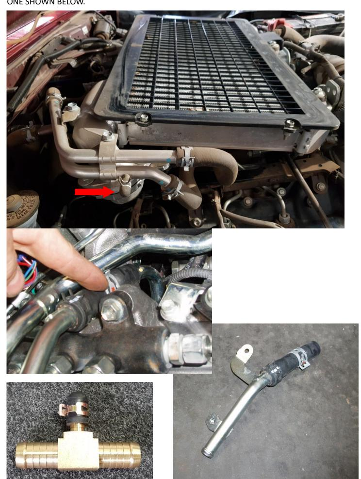
INSTALL HEATER HOSES AS SHOWN. INSTALL THE BRASS T PIECE INTO THE LINE COMING FROM THE FIREWALL USING SUPPLIED HOSE CLAMPS. REUSE THE FACTORY HOSE BLANK AND SECURE WITH SPRING CLIP SUPPLIED (SEE ABOVE PICTURE). RUN SUPPLIED 5/8 HOSE TO MOTOR. INSTALL 1/2-5/8 BRASS JOINER INTO HEATER HOSE RUNNING TO HEATER TAP AND INSTALL 1/2 HOSE AS SHOWN USING SUPPLIED HOSE CLAMPS.
