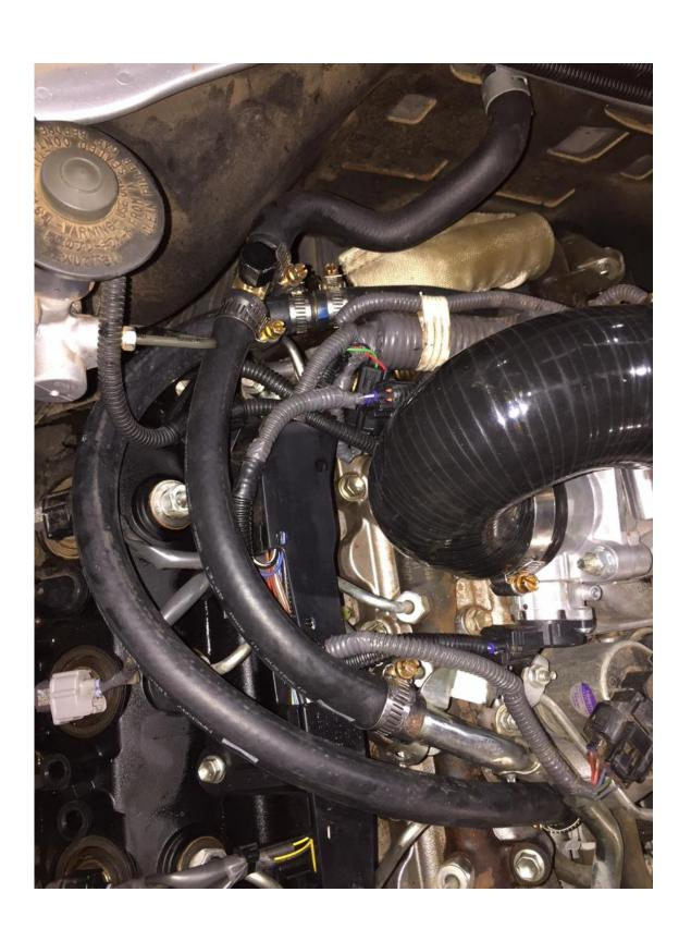
GENTLY TAP DOWN THE BRACKET SHOWN TO ALLOW CLEARENCE TO THE INTERCOOLER.
