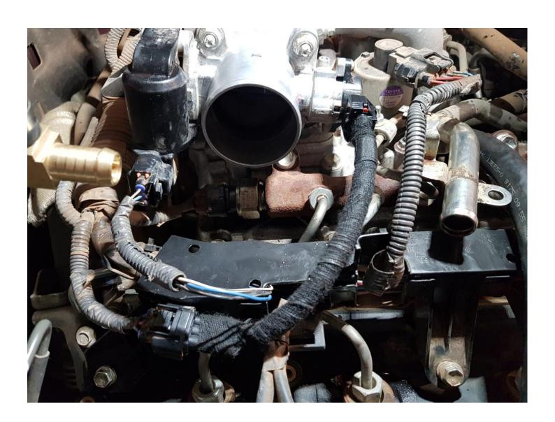
REMOVE THE MOUNTING RUBBERS AND WASHERS (FRONT AND REAR), TEMP SENSOR AND MAP SENSOR INCLUDING SPEED CLIPS FROM THE FACTORY INTERCOOLER. INSTALL THE TEMP SENSOR INTO INLET ADAPTOR USING FACTORY BRASS WASHER. INSTALL MOUNTING RUBBERS TO THE NEW INTERCOOLER FOLLOWED BY THE CRUSH TUBE WASHERS.
