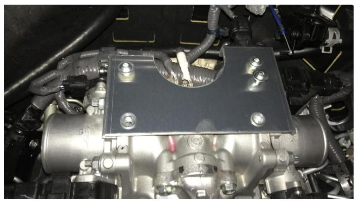
CLEAN THE MANIFOLD INLETS SO NO OIL IS PRESENT. INSTALL THE 180 SILICONE WITH THE SHORTER LEG ON DRIVERS SIDE AS SHOWN (1). THE EQUAL LENGTH 180 TO THE PASSANGER SIDE AND INLET ADAPTOR AS SHOWN WITH THE TEMP BOSS AND LONGER SIDE TO THE PASSANGER SIDE (2) ROTATING AS FAR BACK AS POSSIBLE TIGHTEN HOSE CLAMPS. ORIENTATE SO THE HOSE CLAMPS ARE ABLE TO BE TIGHTENED WITH THE INTERCOOLER FITTED. CONNECT AIR TEMP SENSOR.
