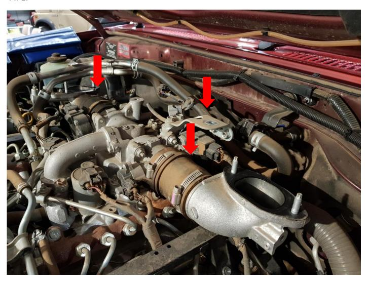
REMOVE MAP SENSOR FILTER AND LOOM FROM THE BRACKET SHOWN AND REMOVE BRACKET.
