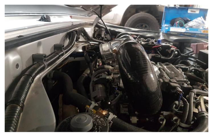
REMOVE THE FACTORY HOSE OFF THE TUBRO PIPE (PASSENGER SIDE). THE BATTERY CAN BE REMOVED FOR BETTER ACCESS.
