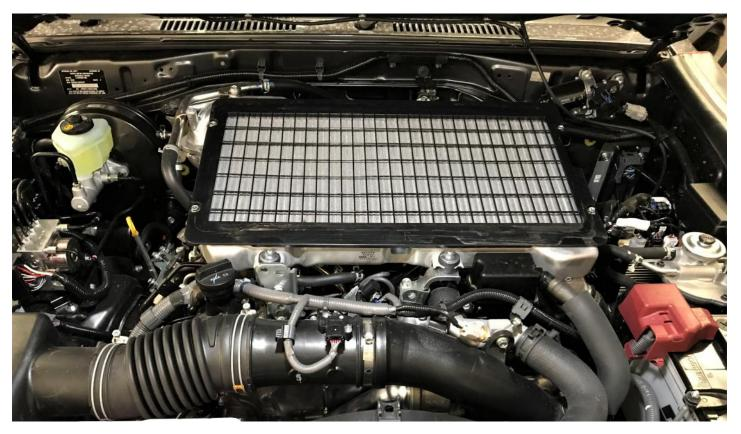
DISCONNECT MAP AND TEMP SENSOR (AT THE REAR OF THE INTERCOOLER). REMOVE FACTORY INTERCOOLER, PIPEWORK TO THE THROTTLE BODIES AND HOSE OFF THE TURBO PIPE.
