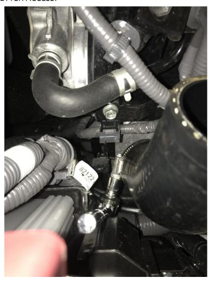
INSTALL STRAIGHT 2" SILICONE HOSE AND INSTALL BOTTOM HOSE CLAMP. INSTALL THE 45 DEGREE ALUMINIUM BEND AND SILICONE, LONG SIDE TO THE INTERCOOLER. PLACE HOSE CLAMPS OVER AND LEAVE PIPEWORK LOOSE.
