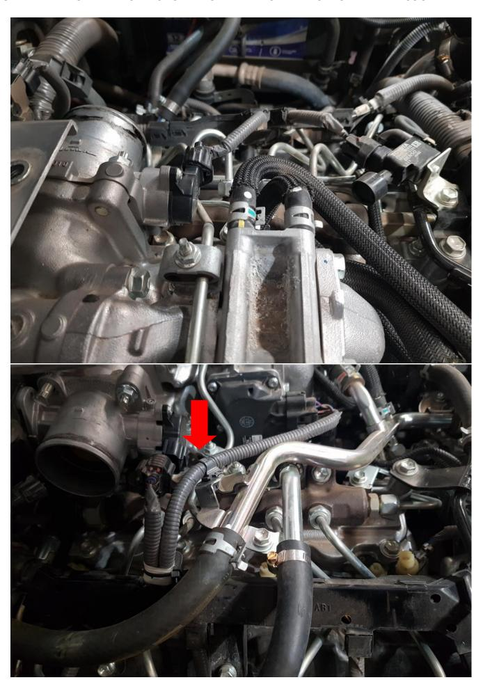
NEXT UNPLUG THE TWO CONNECTORS RUNNING TO THE DRIVERS SIDE THROTTLE BODY. ROTATE THROTTLEBODY 180 DEGREES AND REINSTALL. CONNECT THE EXTENSION LOOM SUPPLIED. THESE ARE VERY TIGHT. USE A PAIR OF PLYERS TO SQUEEZE TOGETHER MAKING SURE YOU HEAR A CLICK. IF NEEDED UNCLIP LOOM COVER AND RUN THE SECOND WIRE OUT THE REAR OF THE LOOM COVER AND CONNECT. RECLIP LOOM COVER.
