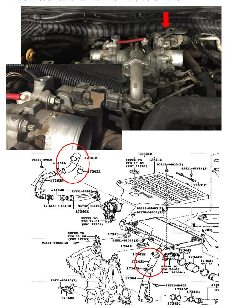
ON ALL MODELS EXCEPT SAHARA UNBOLT HEATER PIPE BRACKET. CLAMP OFF HOSES AT FIREWALL. REMOVE HARDLINE SECTION AND RECONNECT AS SHOWN. IF SAHARA MODIFY HEATER HOSES AFTER MODIFYING DIPSTICK AS SHOWN ON THE FOLLOWING PAGES.
