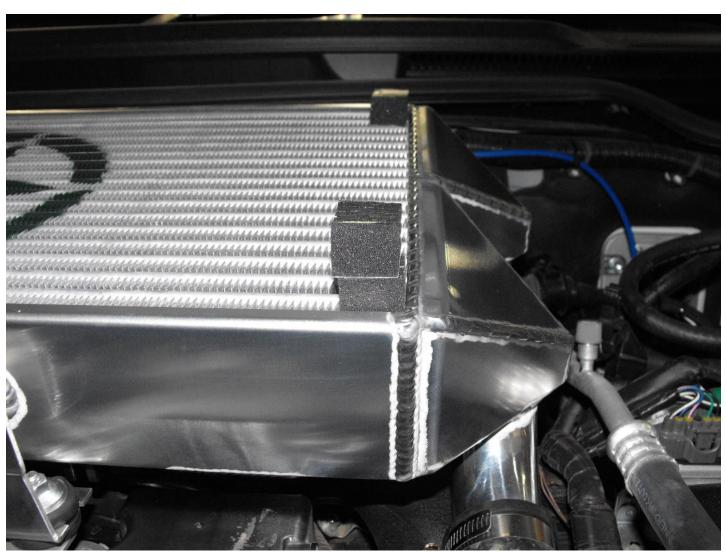
TRIM TO LINE SHOWN FOR APPROPRIATE CLEARENCE TO THE INTERCOOLER THE RIDGES CAN BE CUT BACK ON AN ANGLE FOR ADDED CLEARENCE.
