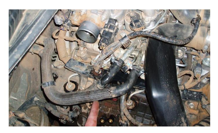
CLEAN THE BASE OF THE DIPSTICK WERE IT ENTERS THE MOTOR. REMOVE DIPSTICK AND HOSE FROM CAR. REMOVE SHORT HOSE AND INSTALL LONG 6MM HOSE SUPPLIED. BOLT TO SUPPLIED BRACKET WITH NUT AND BOLT AND REINSTALL DIPSTICK ROTATED 180 DEGREES.
