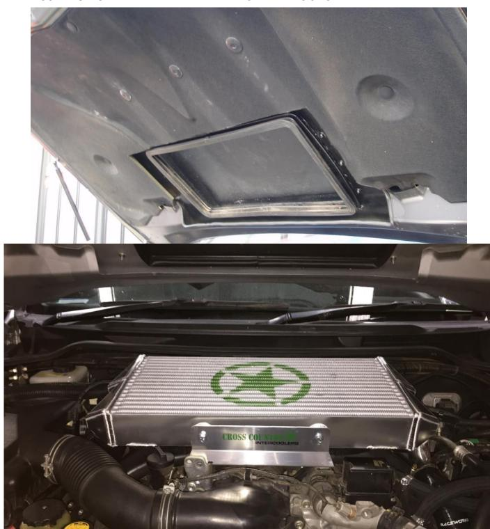
REINSTALL THE BONNET AND RE ATTACH WASHER HOSE. MAKE SURE ALL BOLTS AND HOSE CLAMPS ARE TIGHT. CHECK INTERCOOLER IS TOUCHING THE PINCHWELD AND ADJUST INTERCOOLER IN SLOTS IF NEEDED. CHECK FAN OPERATION AND TEST DRIVE VEHICLE AND CHECK FOR ANY LEAKS.
