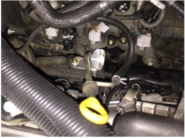
IF SAHARA MODIFY AND INSTALL HEATER HOSES AS SHOWN WITH SUPPLED CLAMPS AND T PIECES.
