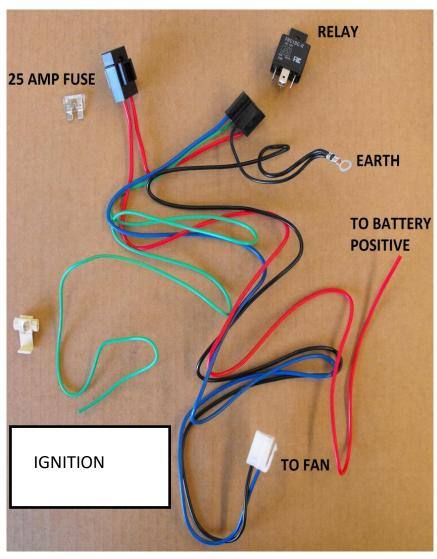
WIRE FANS AS SHOWN BELOW USING THE SUPPLIED WIRING LOOMS AND ADD A FUSE TO PICK UP IGNITION FROM THE FUSE BOX.
