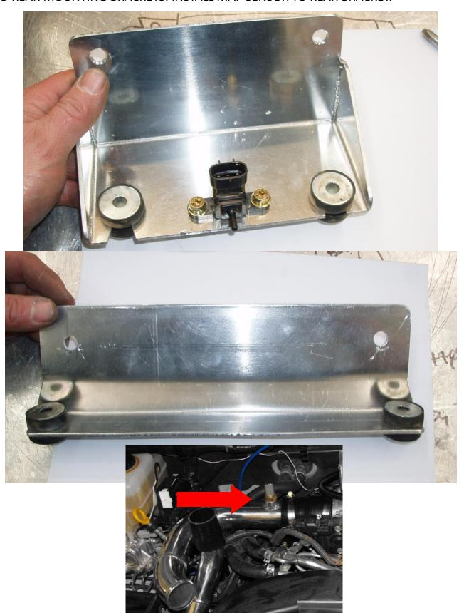
INSTALL FRONT AND REAR BRACKETS USING FACTORY BOLTS AND WASHERS. CONNECT MAP SENSOR AND HOSE. CLEAN THROTTLE BODY INLETS AND TURBO OUTLETS WITH BRAKE CLEANER READY TO FIT THE SILICONE HOSES. INSTALL THE TWO SILICONE REDUCERS AS SHOWN AND TIGHTEN HOSE CLAMP ON THE THROTTLE BODY END. INSTALL 45MM 45 DEGREE SILICONE (80X60) TO THE DRIVERS SIDE TURBO PIPE WITH LONG END TO TURBO FOLLOWED BY THE 45MM 45 DEGREE ALUMINIUM BEND WITH LONG SIDE TO TURBO END. INSTALL HOSE CLAMPS. LEAVE LOOSE.
