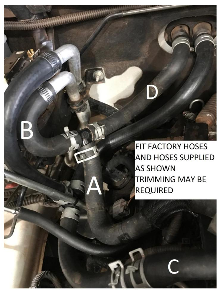
WHEN RE INSTALLING USE SUPPLIED BRASS T PIECES AND HOSE CLAMPS
