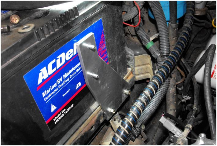
BOLT SUPPLIED POWER STEERING RESERVOIR TO NEW BRACKET. CONNECT SMALL LINE AND USE SUPPLIED 5/8 HOSE TO CONNECT RESERVOIR TO POWER STEERING PUMP.
