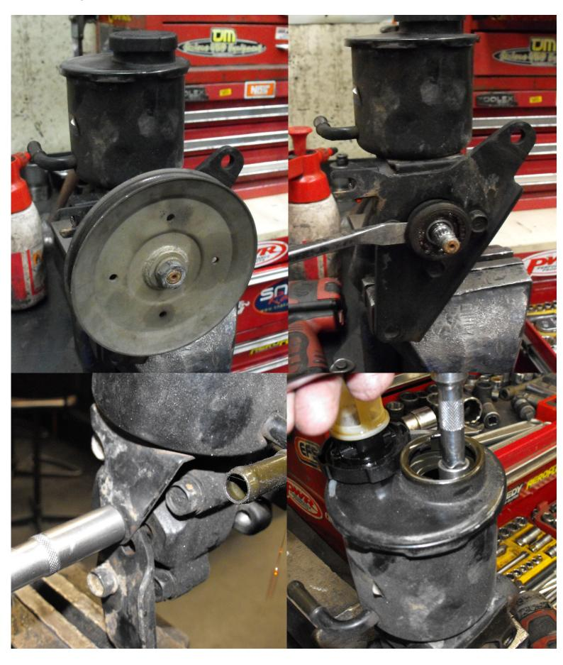
INSTALL SUPPLIED FITTING AS SHOWN USING THE O RING AND TWO M8 NUTS SUPPLIED. RE INSTALL THE POWER STEERING PUMP TO THE CAR. IF MORE CLEARENCE IS NEEDED TO CLEAR THE PIPEWORK FOR THE PLENUM A LONGER BELT CAN BE USED.
