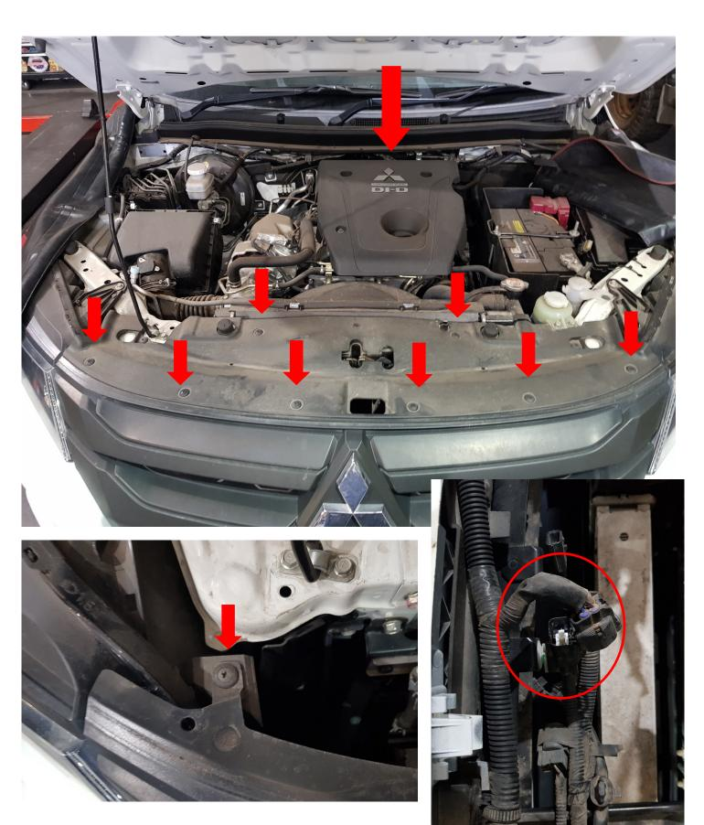
WITH THE FLARES REMOVED START REMOVEL OF THE BUMPER. MQ MODELS UNDO THE THREE SCREWS HOLDING THE BUMPER AND POP THE SIDES OF THE BUMPER FROM THE GUARD. MR MODELS REMOVE NUMBER PLATE AND PLASTIC TRIM BELOW THE FOG LIGHTS AND UNDO ALL SCREWS. POP OUT THE SIDE OF THE BUMPER AND REMOVE.
