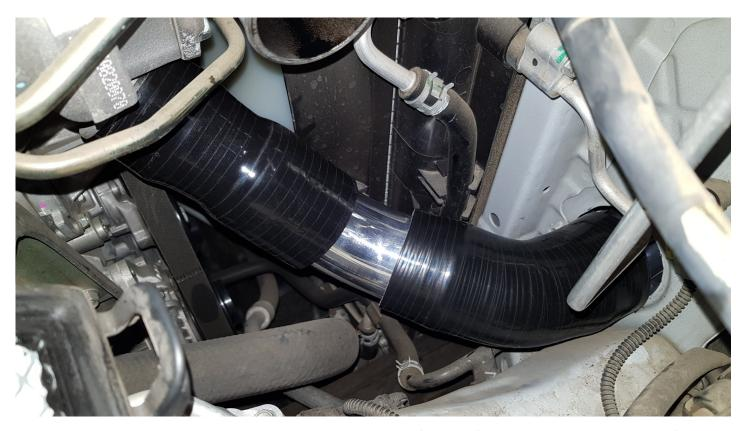
INSTALL THE MANIFOLD SIDE PIPEWORK USING THE 2 3/4" - 2 1/2" STRAIGHT REDUCER, 2 1/2" ALUMINIUM PIPE (53 DEGREE END TO MANIFOLD AND 45 DEGREE END TOWARDS THE INTERCOOLER AND THE 2 1/2" 45 DEGREE SILICONE WITH THE SHORT END TO THE INTERCOOLER. USING THE 1X HS44 AND 3X HS40 HOSE CLAMPS.
