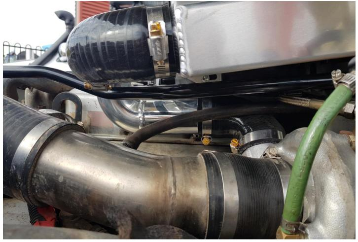
CLEAN THE MATING SURFACE ON THE INTAKE MANIFOLD AND INSTALL INLET ADAPTOR SUPPLIED AS SHOWN USING A SILICONE SEALENT (NOT SUPPLIED). INSTALL 2 1/2" PIPEWORK AS SHOWN LEAVING LOOSE WITH HOSE CLAMPS. IF APPLICABLE RUN A HOSE FOR BOOST REFERENCE TO THE FUEL PUMP. IF NOT BLANK FITTING.
