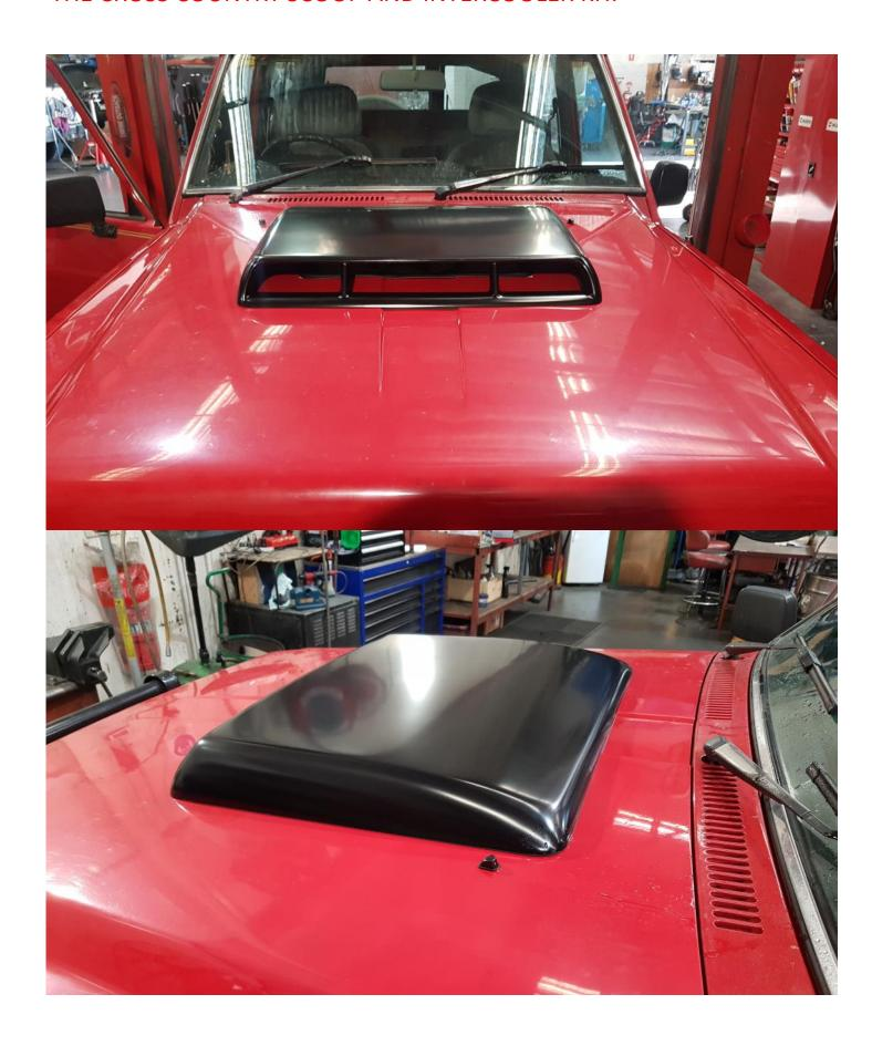
WITH SCOOP FITTED RE INSTALL THE BONNET AND CONNECT THE WASHER HOSE. CHECK THE FAN OPERATION. CHECK ALL HOSE CLAMPS AND FASTENERS ARE TIGHT AND TEST DRIVE THE VEHICLE.
