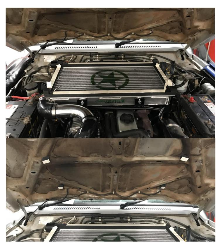
READ THE SCOOP FITING INSTRUCTIONS SUPPLIED WITH THE SCOOP (ALSO BELOW). CUT OUT THE UNDERBONNET WEBBING AS SHOWN. NOTE CUT OUTS
