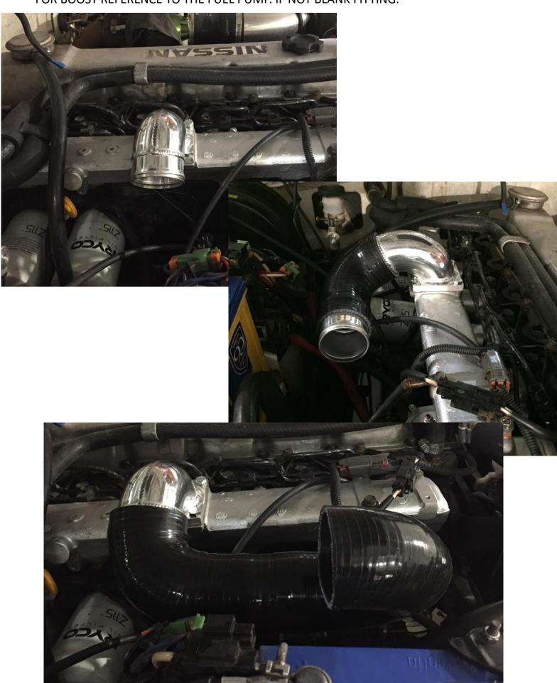
LOOSEN THE REAR CLAMPS ON THE FRAME. FIT INTERCOOLER TO CAR SITTING THE REAR OF THE FRAME ON THE FIREWALL LIKE SHOWN PUSHING TURBO SIDE SILICONE ON AT THE SAME TIME. REINSTALL RADIATOR BOLTS THROUGH THE FRONT OF THE FRAME AND TIGHTEN. TIGHTEN FRAME CLAMPS TO FIREWALL. FIT MANIFOLD SIDE PIPEWORK AND TIGHTEN ALL HOSE CLAMPS.
