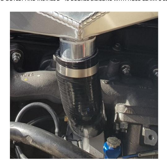
HIGHMOUNT VARIANTS TRIM AND INSTALL PIPEWORK LIKE SHOWN. THE TURBO HOUSING MAY NEED TO BE ROTATED. THE INTERCOOLER MAY NEED TO BE TEST FITTED TO WORK OUT HOSE CUT LENGTH.
