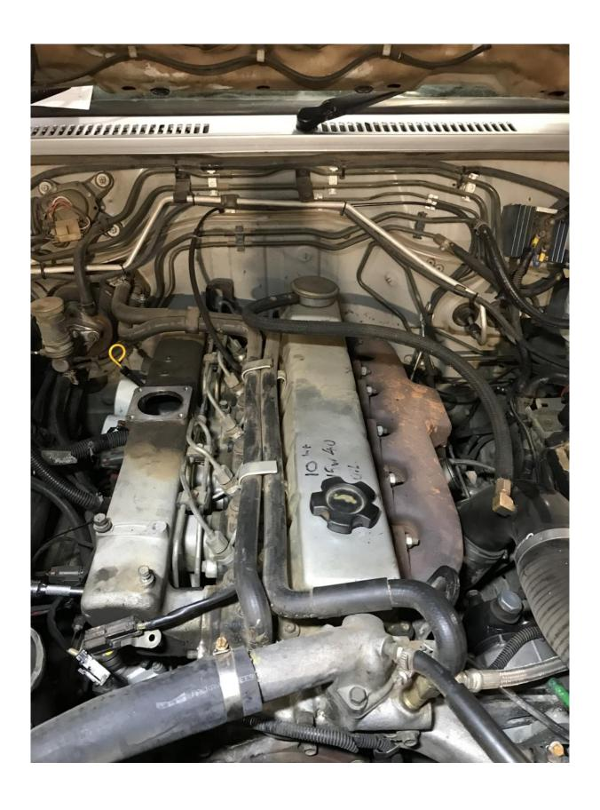
IF THE VEHICLES FUEL FILTER ASSEMBLY IS LOCATED ON THE DRIVERS SIDE IT WILL NEED TO BE MOVED SLIGHTLY FOR CLEARENCE. AN EASY WAY TO DO THIS IS TO RE DRILL THE MOUNTING HOLES ON THE PRIMER HOUSING TO MOVE IT TOWARDS THE GUARD FOR CLEARENCE TO THE INTERCOOLER.
