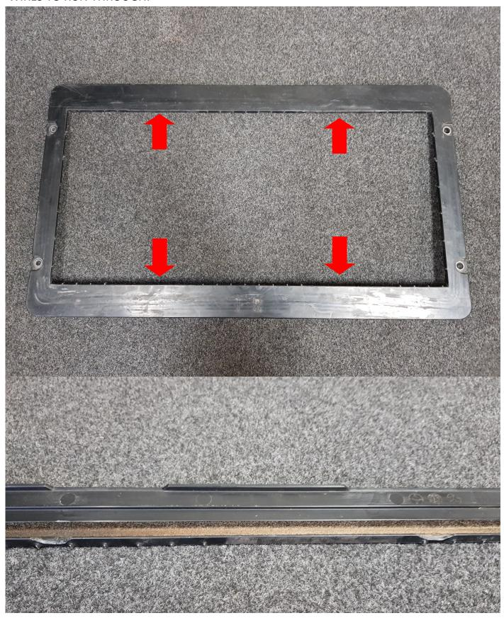
GRIND THE FOUR MOUNTING POINTS DOWN AS SHOWN. GRIND CAREFULLY AS TOO MUCH HEAT IN THE METAL CRUSH TUBE WILL MELT THE PLASTIC AND THE CRUSH TUBE MAY MOVE.
