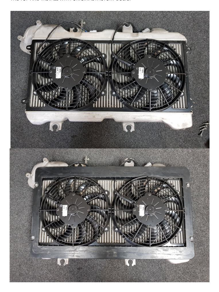
WITH THE FAN KIT INSTALLED WIRE THE SUPPLIED WIRING LOOMS AS SHOWN. A GOOD PLACE FOR IGNITION IS THE BREAK OUT BOX OR WIPER MOTOR. SEE PICS BELOW.
