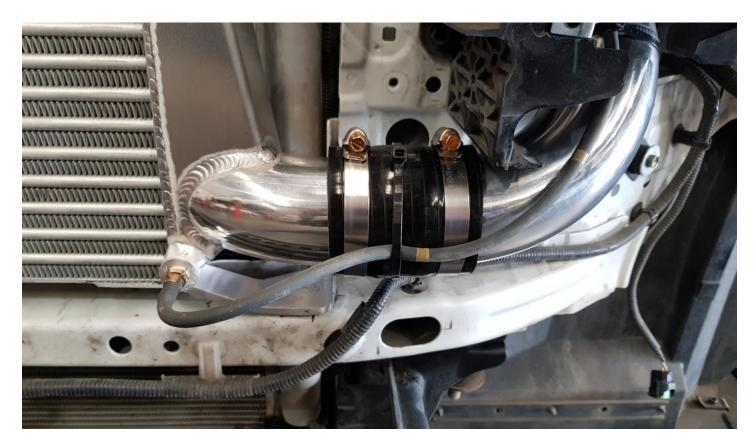
MANOEUVER PIPE WORK AND AIRCON LINES SO THERE IS CLEARENCE TO THE LIGHTS AND BODY WORK. WHEN HAPPY WITH THE FITMENT TIGHTEN PIPE SUPPORT BRACKETS AND HOSE CLAMPS.
