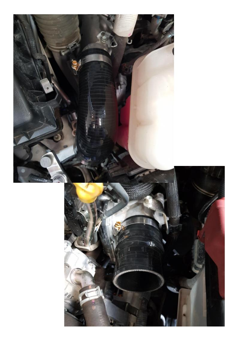
REMOVE TEMP SENSOR FROM FACTORY ELBOW AND INSTALL IN THE MANIFOLD PIPE.
