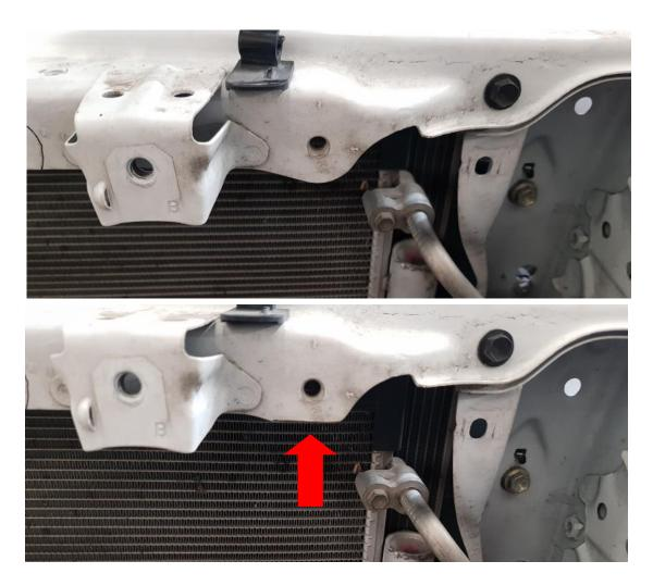
TRIM AS SHOWN. ONCE TRIMMED. LOSEN BOLTS HOLDING THE CENTRE RADIATOR SUPPORT PIECE SO THE INTERCOOLER CAN BE INSTALLED.
