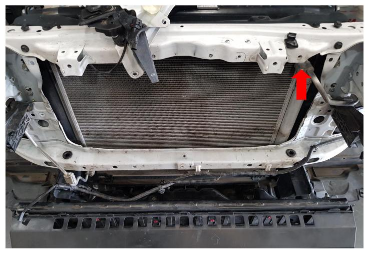
REMOVE GRILL, BUMPER, PLASTIC REINFORCING, HORNS, SIDE DUCTING, FACTORY INTERCOOLER AND PIPEWORK. MARK BONNET CATCH AND UNBOLT AND PLACE OUT OF THE WAY.
