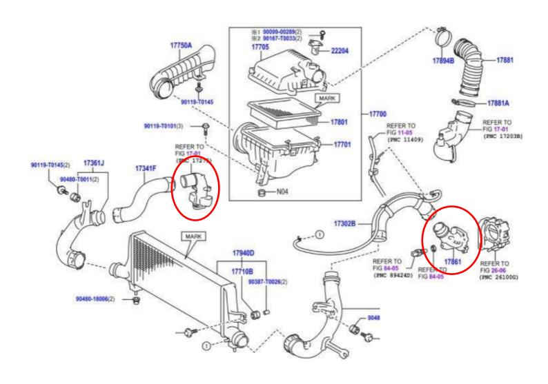
REMOVE TURBO OUTLET PIPE AND REPLACE WITH SUPPLIED ADAPTOR. 2– 2 1/2" 90 DEGREE REDUCER TO THE TURBO OUTLET. TIGHTEN HOSE CLAMPS.
