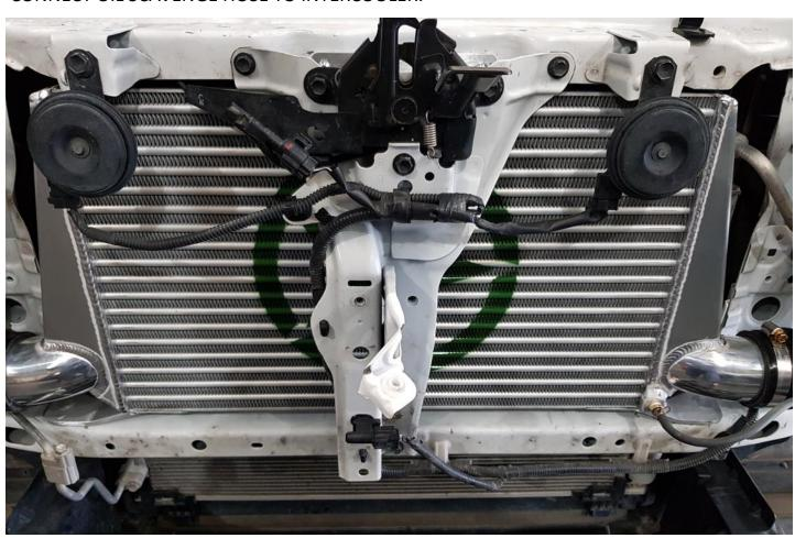
TRIM DUCTING BOTH SIDES TO CLEAR NEW PIPE WORK AND INSTALL. REINSTALL PLASTIC SUPPORT .
