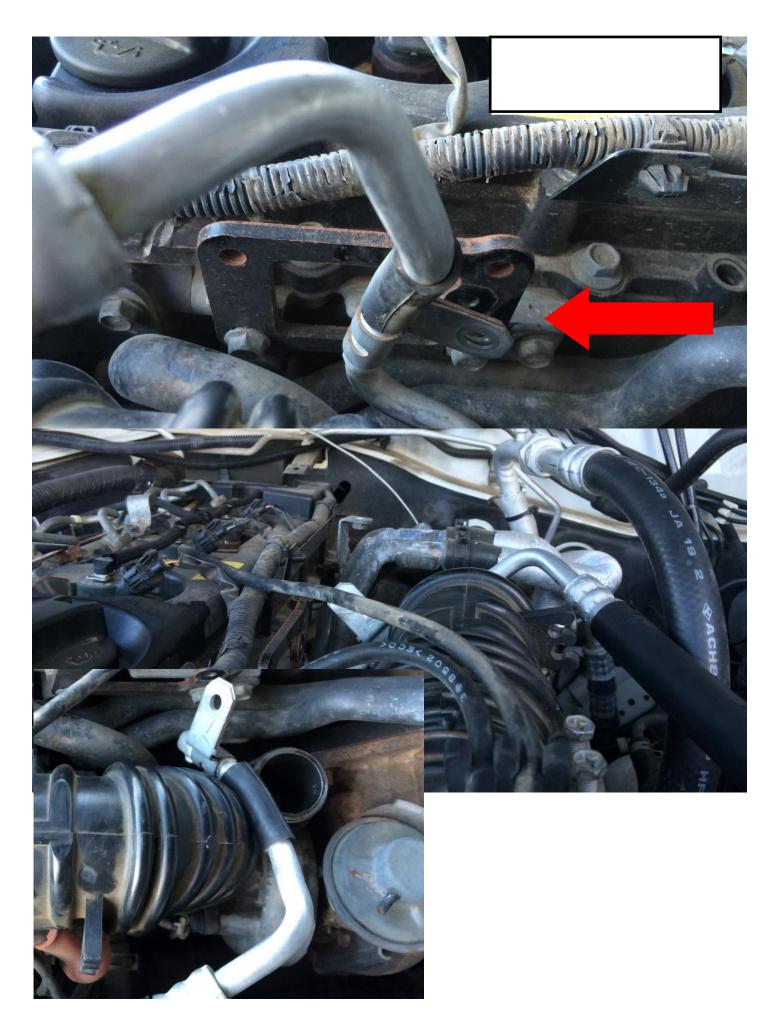
USING A PRY BAR LIKE SHOWN SUPPORT THE AC LINE AT THE FIREWALL (NOT ON THE PIPE IT-SELF BUT THE CONNECTING BLOCK). CAREFULLY PULL THE AC PIPE TO THE PASSANGER SIDE OF THE VEHICLE UNTIL SUFFICIENT CLEARENCE FOR THE INTERCOOLER IS ACHIEVED. THE AC LINES VARY BETWEEN VEHICLES AND MAY BE DIFFERENT TO SHOWN. BE EXTRA CAREFULL IF THE CAR IS FITTED WITH REAR AIR.
