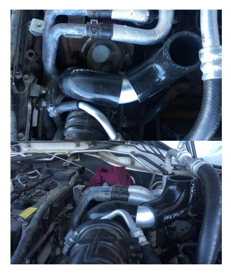
REMOVE MAP SENSOR FROM THE FACTORY INTERCOOLER AND INSTALL ON THE BRACKET ON THE FRAME USING THE FACTORY BOLTS AND SUPPLIED NUTS. RUN THE SUPPLIED BOOST HOSE FROM THE FITTING ON THE INTERCOOLER TO THE MAP SENSOR.
