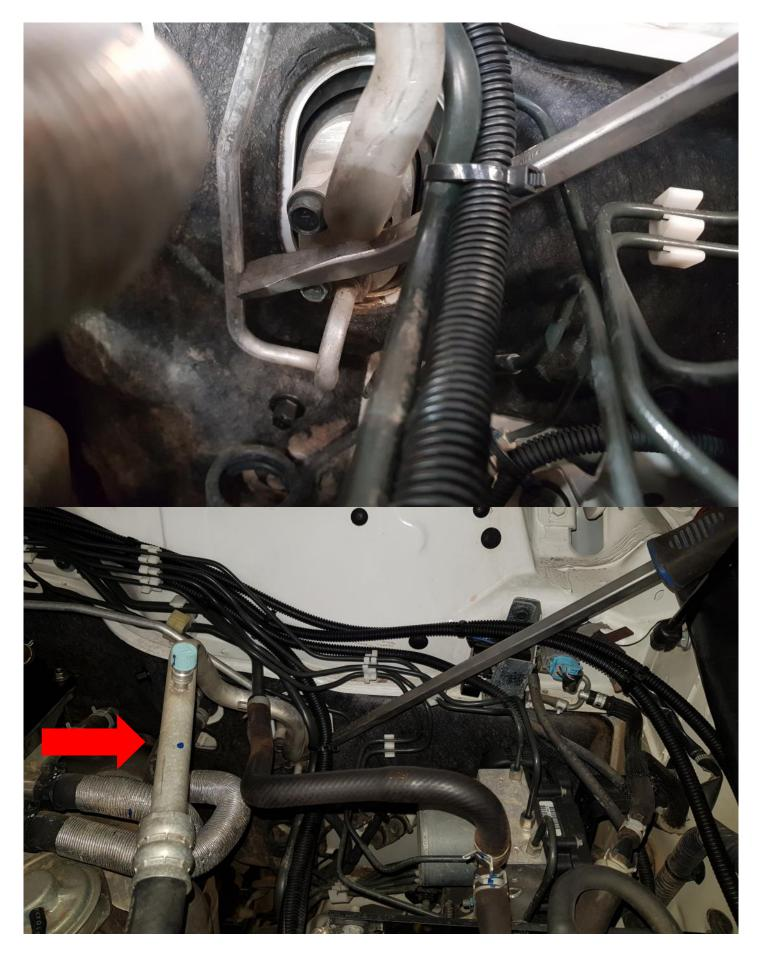
INSTALL STRAIGHT SILICONE REDUCER TO INTAKE MANIFOLD. THIS IS VERY TIGHT. SLIDE HOSE CLAMPS OVER. TIGHTEN HOSE CLAMP ON MANIFOLD LEAVE THE OTHER LOOSE. IN-STALL ALUMINIUM PIPE AS SHOWN. INSTALL 45 DEGREE SILICONE AS SHOWN. SLIDE HOSE CLAMPS OVER AND LEAVE LOOSE.
