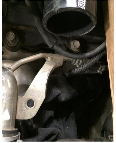
INSTALL PIPEWORK AS SHOWN. INSTALL THE LONGEST LEG 1 3/4" SILICONE TO THE TURBO OUTLET. AND THE SHORTEST LEG 2 1/4" SILICONE TO THE INTERCOOLER INLET. RUN SUPPLIED 4MM HOSE FROM MAP SENSOR TO THE FITTING ON THE INTERCOOLER PIPEWORK. REINSTALL THE INTERCOOLER CONNECTING THE SILICONE HOSES. ONCE FITTED AND ADJUSTED TIGHTEN ALL HOSE CLAMPS.
