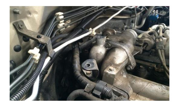
REMOVE BRACKET SHOWN AND UN BOLT SOLENOIDS. THE VACUUM LINES CAN BE PERISHED. CHECK CAREFULLY.
