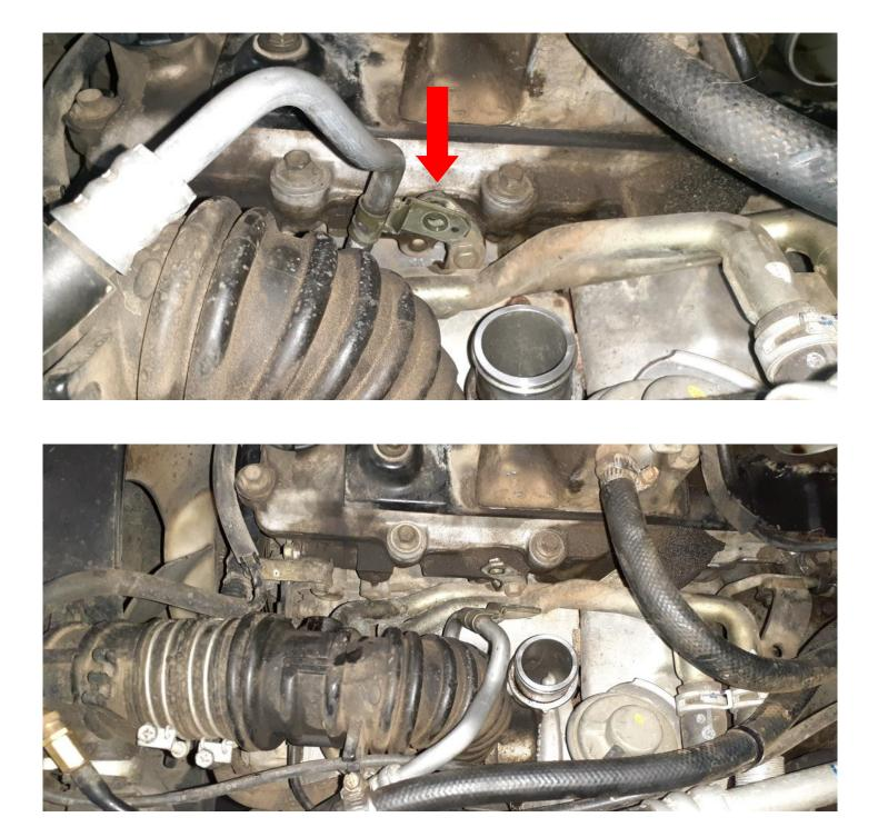
USING A PRY BAR LIKE SHOWN SUPPORT THE AC LINE AT THE FIREWALL (NOT ON THE PIPE ITSELF BUT THE CONNECTING BLOCK). CAREFULLY PULL THE AC PIPE TO THE PASSANGER SIDE OF THE VEHICLE UNTIL SUFFICIENT CLEARENCE FOR THE INTERCOOLER IS ACHIEVED. THE AC LINES VARY BETWEEN VEHICLES AND MAY BE DIFFERENT TO SHOWN. BE EXTRA CAREFUL IF THE CAR IS FITTED WITH REAR AIR.
