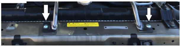
WITH A GRINDER REMOVE MATERIAL FROM THE HEATER HOSE SUPPORT BRACKET (REAR PASSANGER SIDE) AS SHOWN FOR CLEARNCE FOR THE INTERCOOLER PIPEWORK.
