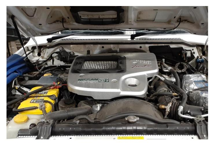
REMOVE BRACKET FROM TOP OF MANIFOLD FOR CLEARENCE TO THE INTERCOOLER.
