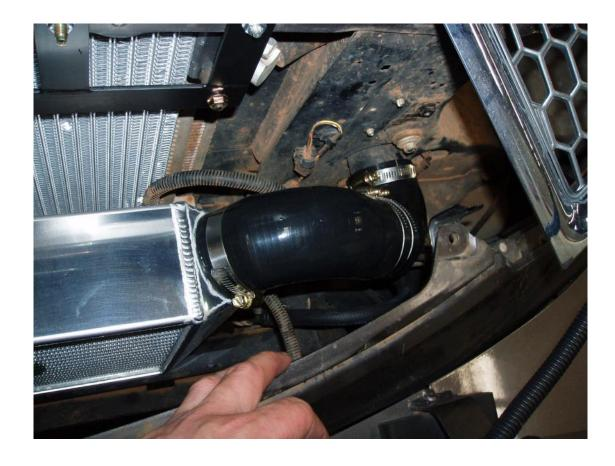
**Step 6** It will now be necessary to trim the two plastic headlight/grille supports that sit either side of the cooler just under the headlights for clearance to the intercoolers pipe work. Please see picture below
