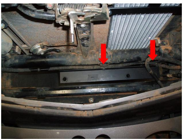
WHEN INSTALLING THE INTERCOOLER CHECK THERE IS CLEARENCE TO THIS BRACKET (PASSENGER SIDE).
