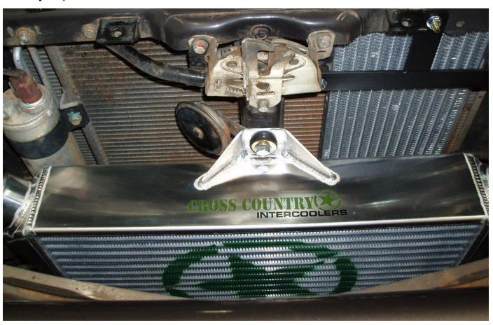
**Step 5** Fit supplied hard pipe (aluminium) and silicon elbow to the R/H side of the cooler and turbo outlet hose. Before tightening clamps, be sure there is adequate clearance around the hard pipe where it passes through the radiator support panel. Once satisfied with the position of the pipe, tighten hose clamps.
