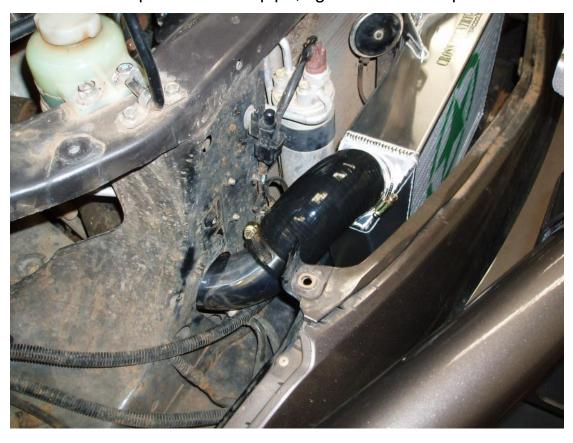
Then fit the supplied L/H side silicon pipe to the intercooler and the factory steel pipe protruding through the radiator support panel. Tighten clamps.
