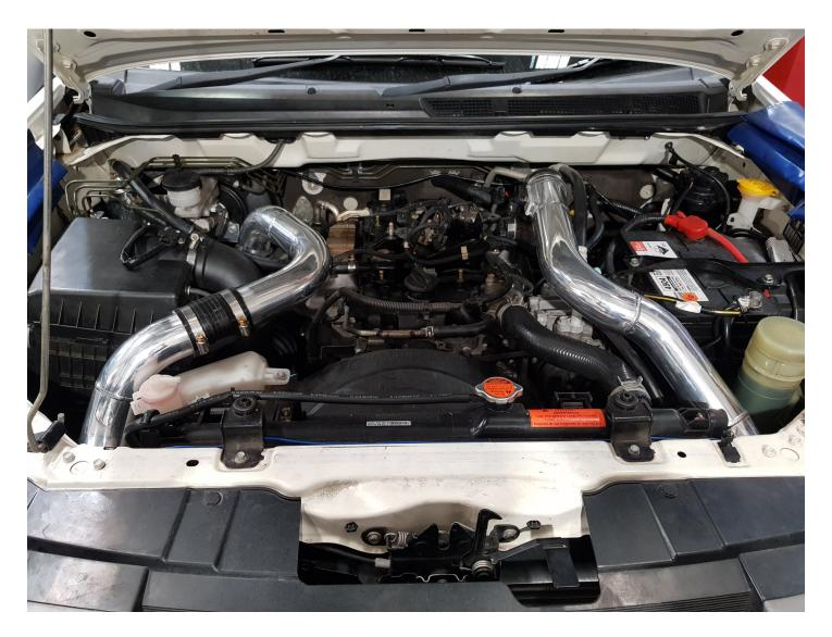
THE ENGINE COVER WILL NEED TO BE TRIMMED BOTH SIDES TO ALLOW CLEARENCE FOR THE NEW PIPEWORK.
