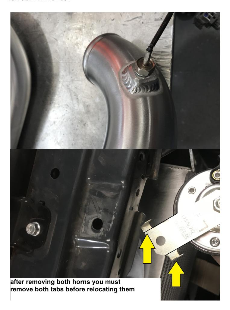
REMOVE FACTORY INTERCOOLER, HORNS AND CENTRE RADIATOR SUPPORT BRACKET AND BONNET LATCH. MARK BONNET LATCH POSITION BEFORE REMOVAL
