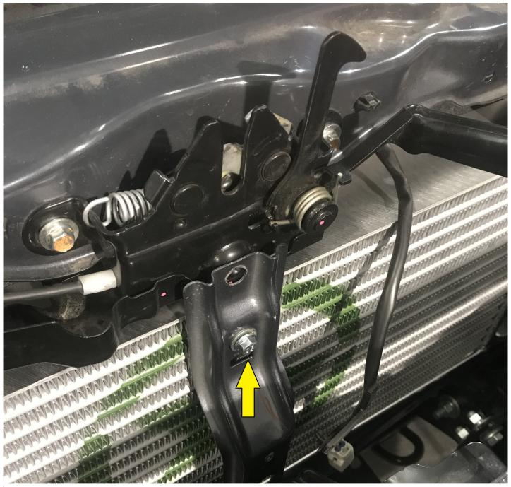
The lower M6 bolt located on the bonnet latch must be replaced with the M6x10 bolt and washer provided.
