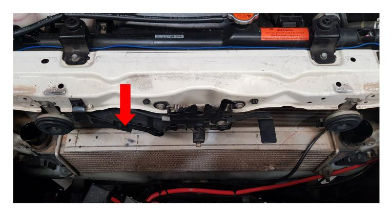
INSTALL INTERCOOLER INTO FACTORY LOWER MOUNTS AND USE 2 PANEL BOLTS SUPPLIED AND MOUNT TO HOLES SHOWN.
