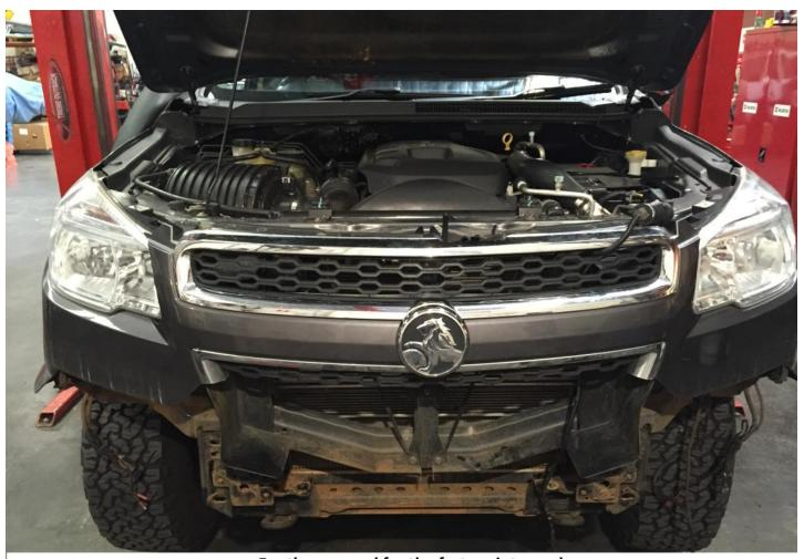
For the removal for the factory intercooler.
