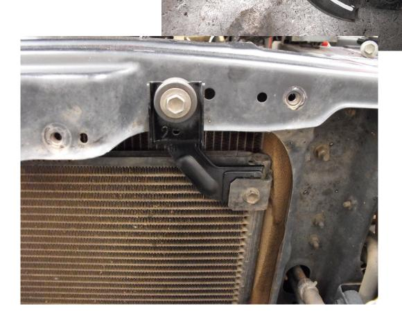
ON SOME VEHICLES THIS PART OF THE RADIATOR PANEL WILL NEED TO BE TRIMMED TO MAKE CLEARENCE FOR THE INTERCOOLER. INSTALL STRAIGHT SILICONE ON THE INTERCOOLER AND TIGHTEN HOSE CLAMP.
