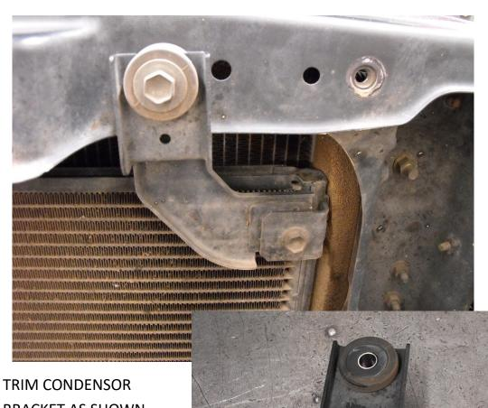
TRIM CONDENSOR BRACKET AS SHOWN. PAINT AND REINSTALL.
