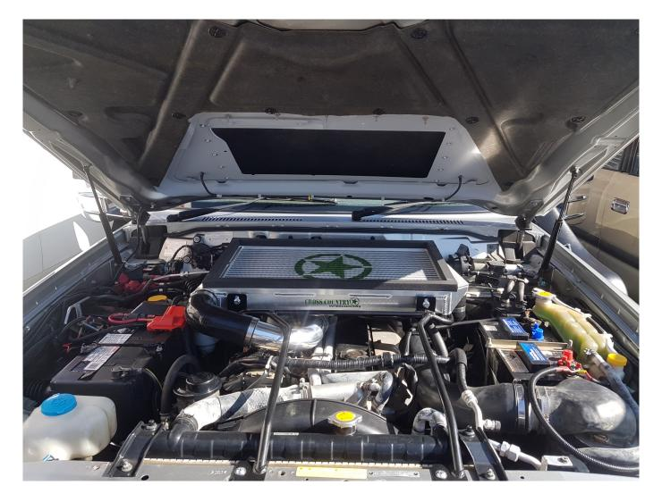
REFIT THE BONNET TO THE CAR AND RE ATTACH WASHER HOSE. MAKE SURE ALL BOLTS AND HOSE CLAMPS ARE TIGHT. CHECK FAN OPERATION AND TEST DRIVE VEHICLE AND CHECK FOR ANY LEAKS.
