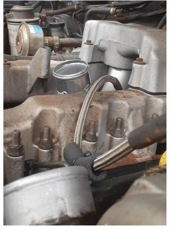
INSTALL THE INTERCOOLER AS SHOWN (THE INTERCOOLER WILL BE REMOVED AGAIN AFTER THE FOLLOWING STEPS). TIGHTEN THE TWO REAR MOUNTING NUTS. MARK THE FRONT MOUNTING HOLES OF THE FRAME TO BE DRILLED. PLACE SUPPLIED FOAM SQUARES STICKY SIDE UP ON THE OUTSIDE EDGES OF THE INTERCOOLER FOAM. GENTLY CLOSE BONNET AND PUSH DOWN. OPEN THE BONNET AND THE FOAM SQUARES WILL HAVE TRANSFERRED TO THE UNDERSIDE OF THE BONNET SHOWING THE LOCATION OF THE INTERCOOLER.
