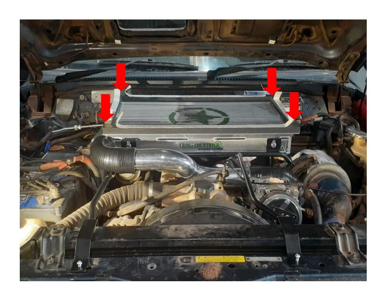
INSTALL PIPE WORK AS SHOWN. THE SILICONES WILL NEED TO BE TRIMMED TO SIZE.
