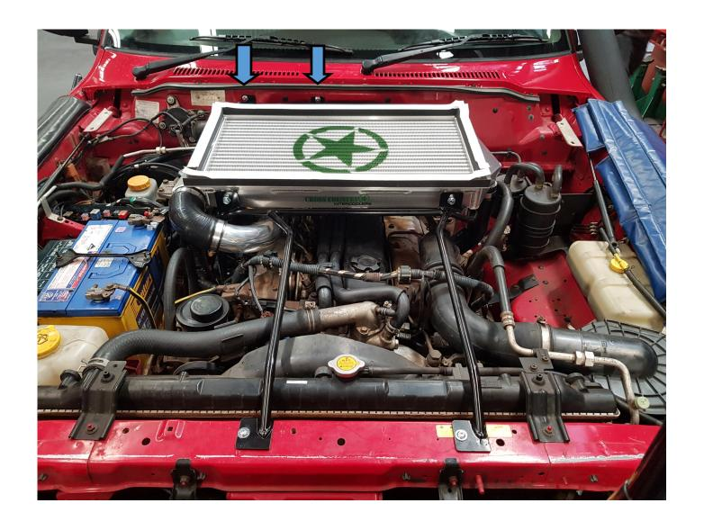
AFTER ADJUSTING AC LINES FIT INTERCOOLER TO REAR STUDS ON THE FIREWALL. TIGHTEN WITH NUTS SUPPLIED. MARK THE TWO FRONT MOUNTING HOLES.
