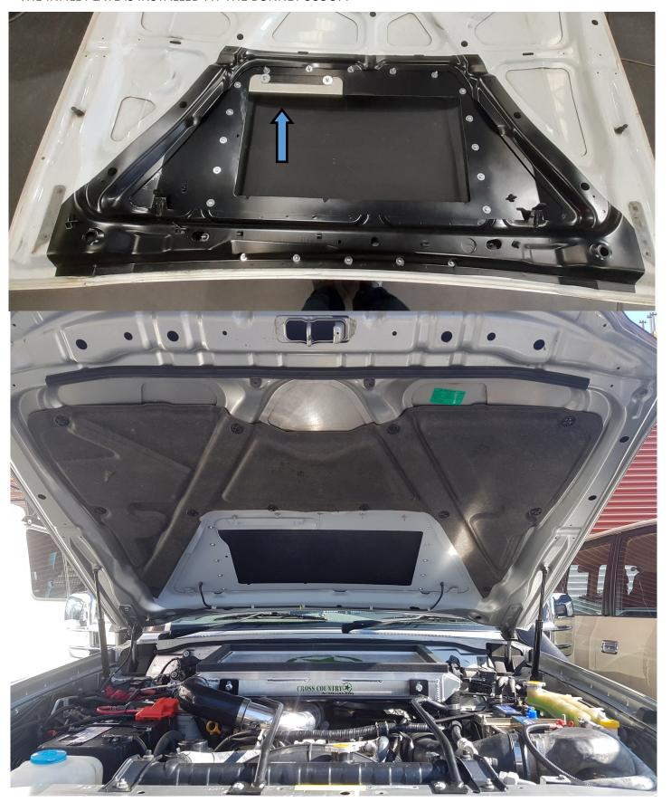
REFIT THE BONNET TO THE CAR AND RE ATTACH WASHER HOSE. MAKE SURE ALL BOLTS AND HOSE CLAMPS ARE TIGHT. CHECK FAN OPERATION AND TEST DRIVE VEHICLE AND CHECK FOR ANY LEAKS.
