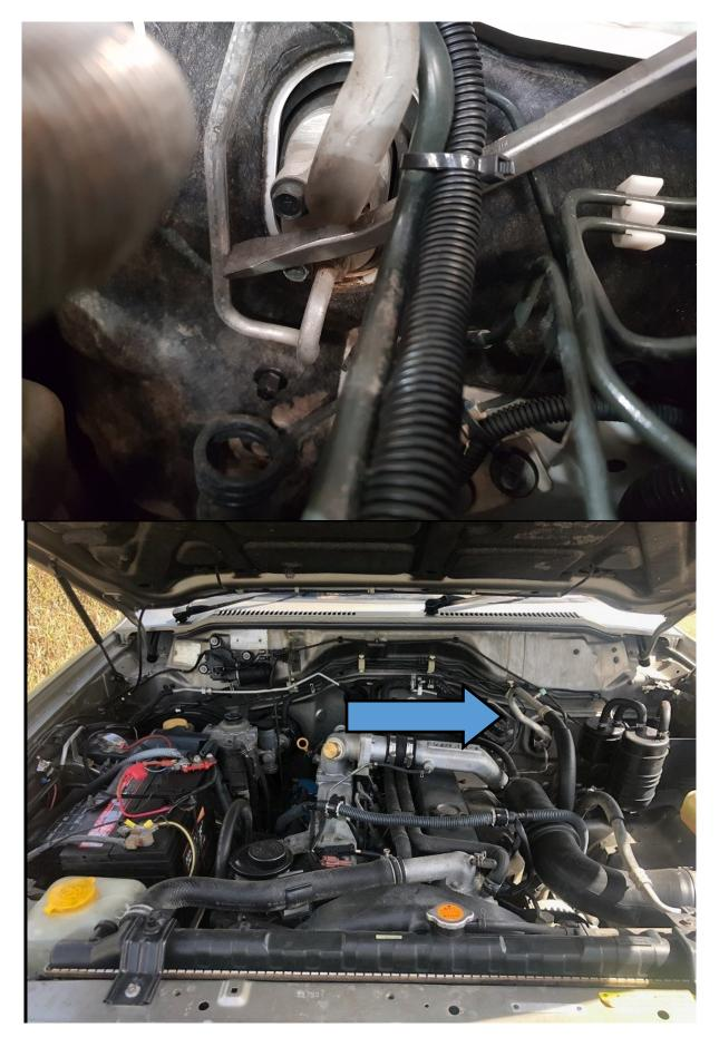
USING A PRY BAR LIKE SHOWN SUPPORT THE AC LINE AT THE FIREWALL (NOT ON THE PIPE ITSELF BUT THE CONNECTING BLOCK). CAREFULLY PULL THE AC PIPE TO THE PASSANGER SIDE OF THE VEHICLE UNTIL SUFFICIENT CLEARENCE IS ACHIEVED. THE AC LINES VARY BETWEEN VEHICLES. MAY BE DIFFERENT TO SHOWN
