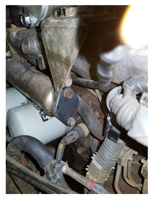
FIT SUPPLIED EGR BLANK TO EGR COOLER USING HIGH TEMP SILICONE SEALANT. IF THE EGR COOLER IS BEING COMPLETELY REMOVED THE BLANK CAN BE USED OF THE EXHUAST MANIFOLD. PLEASE NOTE WE DO NOT SUPPLY ALL THE PARTS TO REMOVE THE EGR COMPLETELY.
