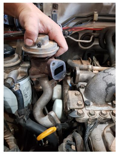
UNBOLT EARTHS, DIPSTICK AND EGR COOLER BRACKET FROM INLET ADAPTOR AND REMOVE INLET ADAPTOR. REMOVE HARDLINE AND BRACKET SHOWN. THE LOOM BRACKET SHOWN MAY NEED TO BE BENT FOR CLEARENCE TO THE INTERCOOLER.
