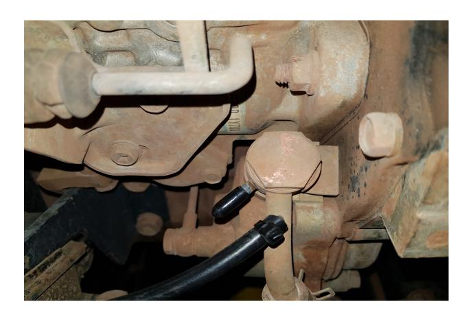
THE SOLENOIDS AND VACUUM LINES FOR THE EGR AND SOFT SHUT DOWN BUTTERFLY CAN BE UN-
