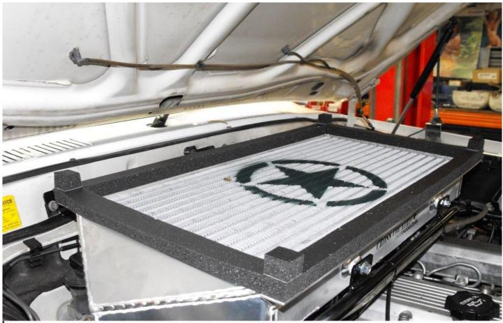
Place one square piece of foam supplied on all four corners of the intercooler and carefully close bonnet until all pieces have stuck to the underside of the bonnet
