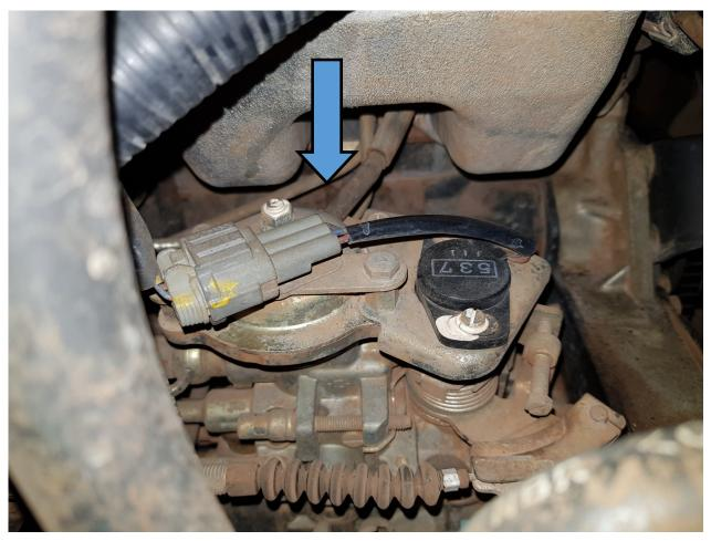
USE SUPPLIED HOSE BLANK TO BLANK THE LINE COMING OFF THE VACUUM PUMP THAT WAS PREVIOUSLY RUNNING TO THE EGR/ SOFT SHUT OFF SOLENOIDS.
