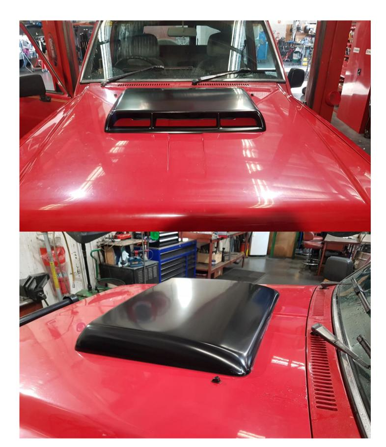
WITH SCOOP FITTED RE INSTALL THE BONNET AND CONNECT THE WASHER HOSE. CHECK THE FAN OPERATION. CHECK ALL HOSE CLAMPS AND FASTENERS ARE TIGHT AND TEST DRIVE THE VEHICLE.
