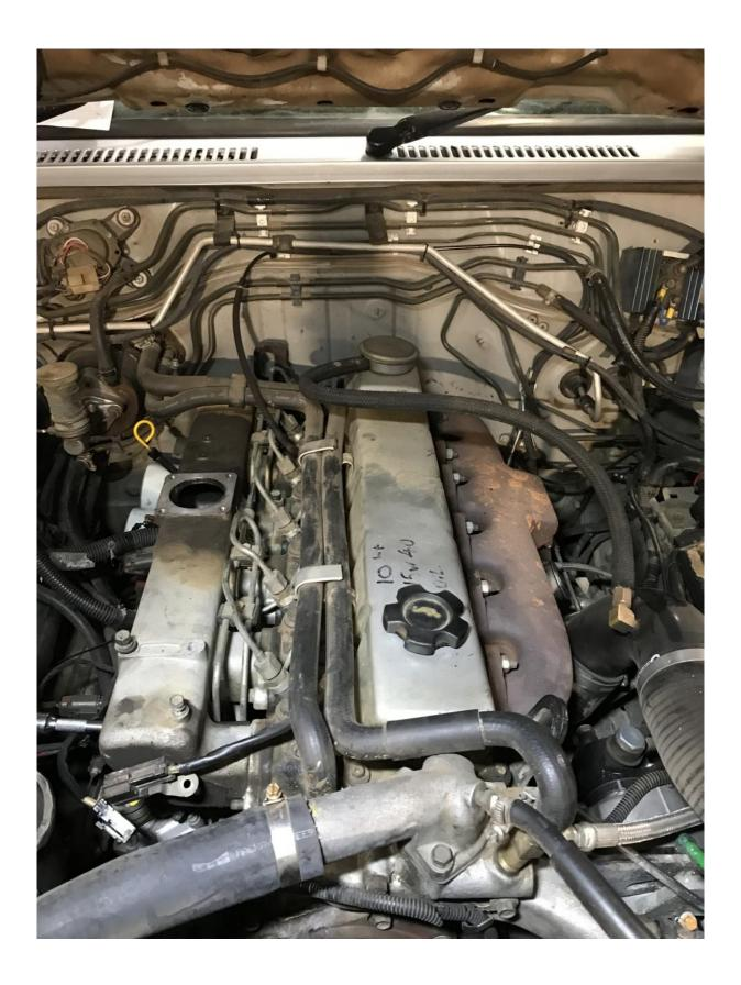
CLEAN THE MATING SURFACE ON THE INTAKE MANIFOLD AND INSTALL INLET ADAPTOR SUPPLIED AS SHOWN USING A SILICONE SEALENT (NOT SUPPLIED). INSTALL 2 1/4" PIPE-WORK AS SHOWN LEAVING LOOSE. IF APPLICABLE RUN A HOSE FOR BOOST REFERENCE TO THE FUEL PUMP. IF NOT BLANK FITTING.
