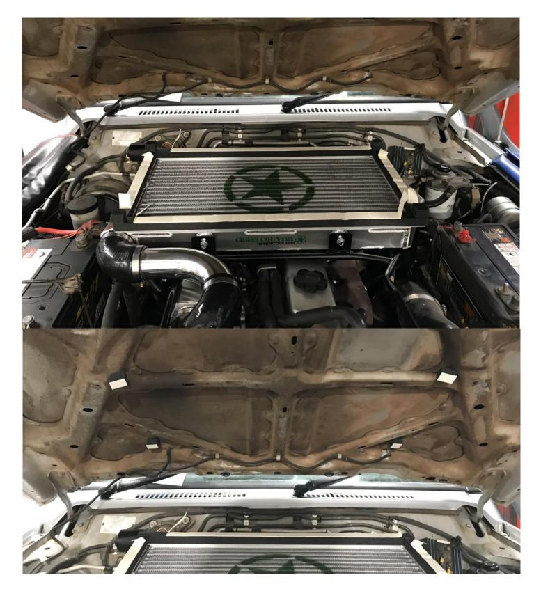
READ THE SCOOP FITING INSTRUCTIONS SUPPLIED WITH THE SCOOP (ALSO BELOW). CUT OUT THE UNDERBONNET WEBBING AS SHOWN.
