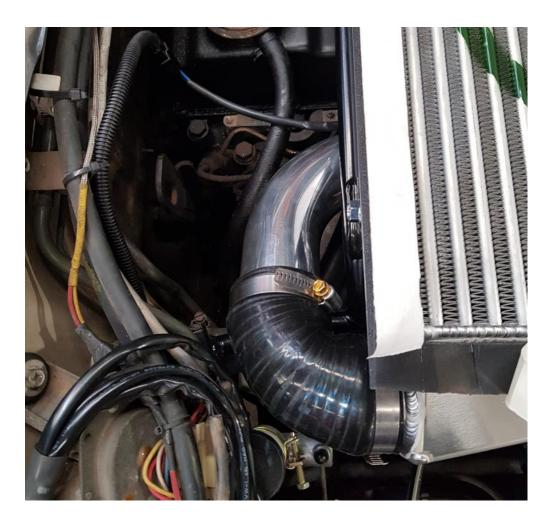
FOR LOW MOUNT TURBO SETUPS TRIM SUPPLIED 2" SILICONES AS SHOWN AND INSTALL USING JOINER AND HOSE CLAMPS. FOR HIGH MOUNT SETUPS CUT AND TRIM SILICONES AS SHOWN USING 2" JOINER AND HOSE CLAMPS. PLEASE NOTE HIIGHMOUNT SETUPS MAY VARY TO THE PICTURE SHOWN.
