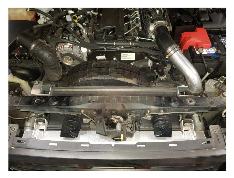
Install horns using brackets shown in position shown on above picture. Reconnect wires.
