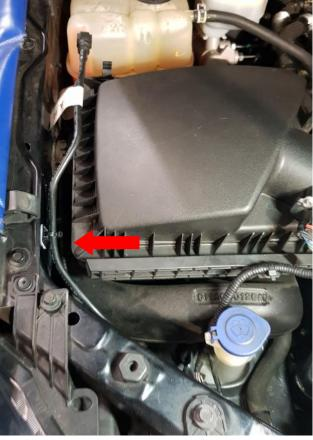
Gently bend the AC to the passenger side of the vehicle to allow clearance for the intercooler pipework. The corner of the fan shroud can be trimmed for clearance if needed.
