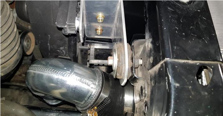
With pipework installed, install turbo pipe support bracket as shown using supplied M8x25 bolt. Reinstall shroud mounting bolts both sides. Adjust large shroud and install with the M6 panel bolts supplied. Reinstall airbox lid and airbox to turbo pipe.
