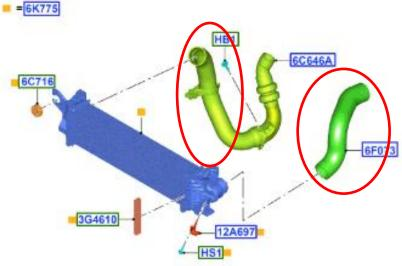
Remove intercooler pipes circled. Leave plastic pipe from turbo attached.
