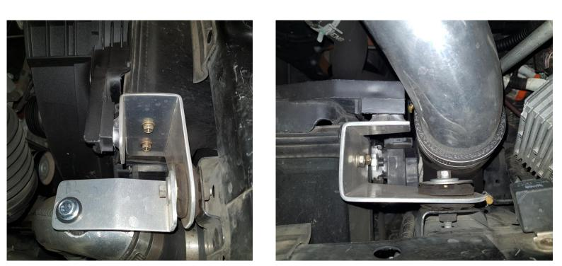
Before installing pipework. Clean the throttle body and lower turbo hose using brake cleaner or similar so no oil is present on the mating surfaces. Locate the 57-63mm 90 degree silicone reducer. Install the 57mm end to the passenger side of the intercooler. Install hose clamps loose. Install the short end of the aluminum bend into the 90 degree reducer slide hose clamps over and install the 63mm 45 degree silicone to throttle body. Adjust and tighten all clamps.
