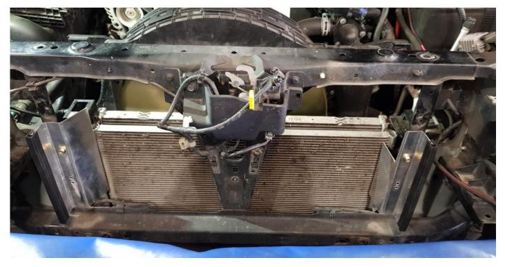
Install the 4 supplied rubbers to the intercooler mounting points. Place the intercooler in position and install the crush tubes followed by the panel washer and m6x40 bolts. Connect the temp sensor wire. This will have to be ran through the same hole as the intercooler pipe on the passenger side.
