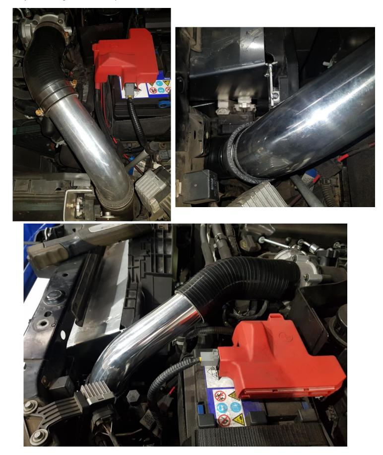
Install the 63-70mm silicone reducer to the factory pipe coming from the turbo. For ease of fitment adjust to approx. position and tighten hose clamp on the 70mm end. Install the short 45 degree 57mm silicone to the intercooler. Install hose clamps loosely. Install the aluminum pipe between the two. Loosen lower hose clamp and adjust pipework and tighten all hose clamps.
