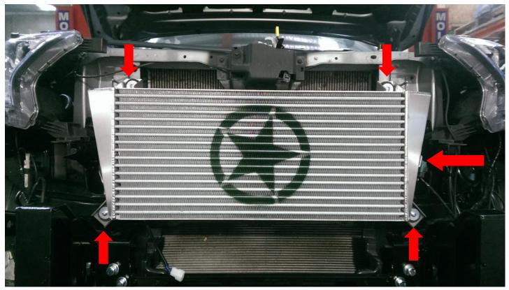
For clearance to the intercooler pipework the return line from the radiator to overflow bottle will need to be unclipped and secured into place using supplied cable ties and adhesive mounts
