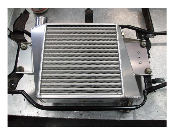
BEFORE INSTALLING THE INTERCOOLER, CLEAN THE INSIDE ENDS OF THE PIPEWORK WITH A SOLVENT LIKE BRAKE CLEANER TO REMOVE OIL RESIDUE.
