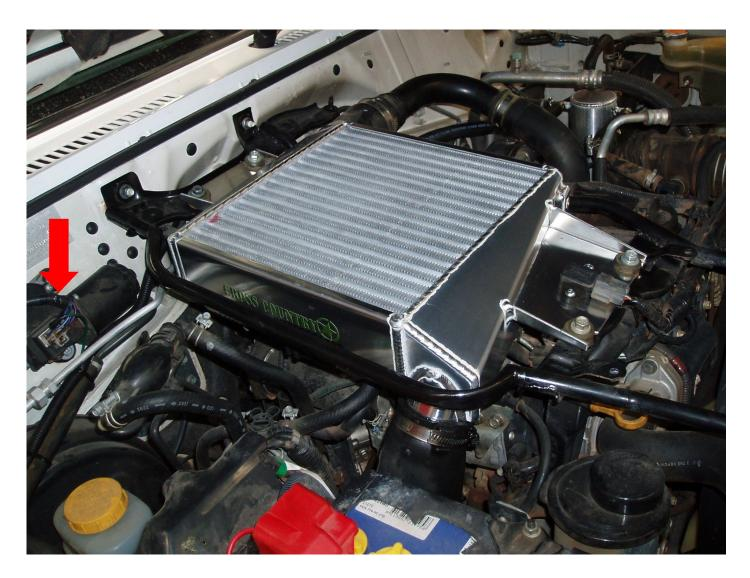
WITH THE INTERCOOLER INSTALLED. TEST DRIVE VEHICLE.
