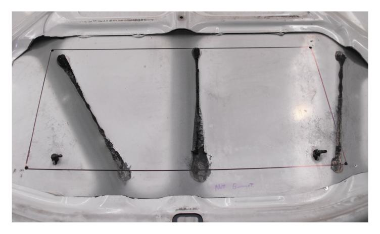
THE WASHER JETS NEED TO BE MOVED OUTWARDS 50MM FROM THE SCOOP BOLT HOLES IN LINE WITH ORIGINAL WASHER JETS
