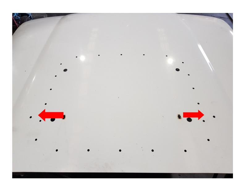
AFTER PAINTING AND INSTALLING THE SCOOP INSTALL THE WASHER JETS AND HOSE SUPPLIED.
