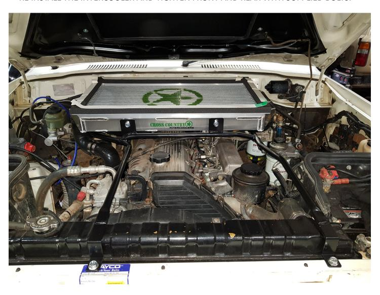
INSTALL MANIFOLD PIPEWORK AS SHOWN. THE SILICONE WILL NEED TO BE TRIMMED. ONCE INSTALLED TIGHTEN HOSE CLAMPS.
