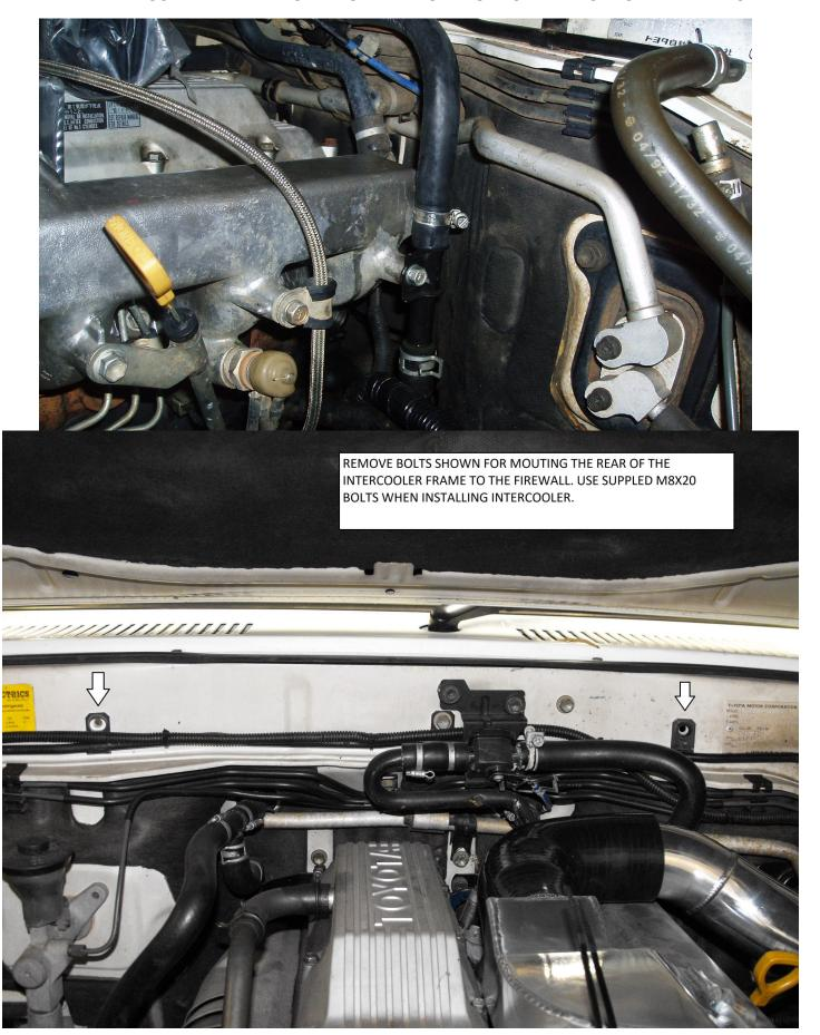
CLEAN SURFACES AND INSTALL INLET ADAPTOR USING SILICONE SEALENT AND REBOLT THROTTLE CABLE BRACKET TO ADAPTOR. RUN THE VAC LINE FROM FITTING ON THE INLET ADAPTOR (NOT SHOWN) TO THE BOOST LINE T PIECE OR FUEL PUMP.
