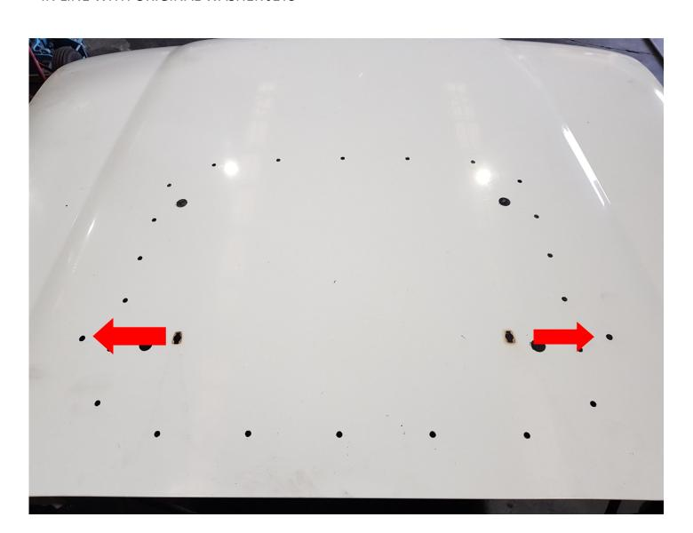
AFTER PAINTING AND INSTALLING THE SCOOP INSTALL THE WASHER JETS AND HOSE SUPPLIED.
