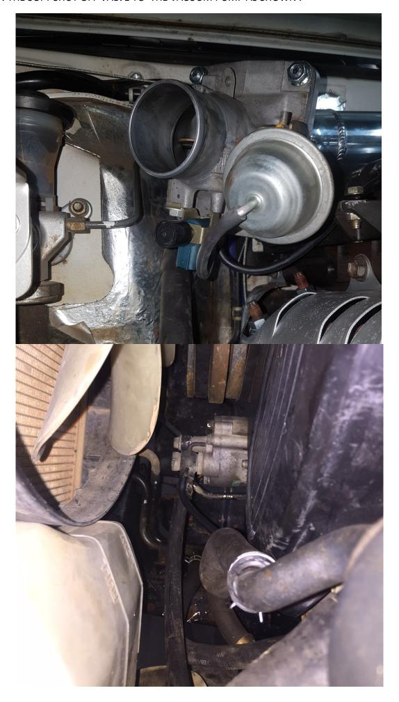
IF A 100 SERIES 1HDFTE MOTOR IS FITTED THE POWER STEERING BRACKET WILL NEED TO BE MODIFIED AS SHOWN TO ALLOW CLEARENCE TO THE INTERCOOLER PIPE WORK.
