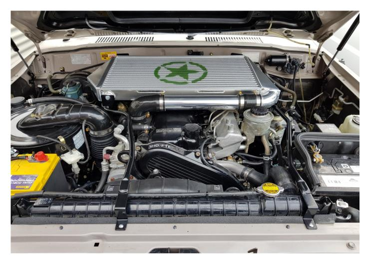
START WITH THE REMOVAL OF THE FACTORY UNDER BONNET SOUND DEADENING FOLLOWED BY THE CROSS OVER PIPE, SILICONE AND TURBO PIPE. REMOVE EGR PIPE. REMOVE THE STEEL ROCKER COVER COVER.
