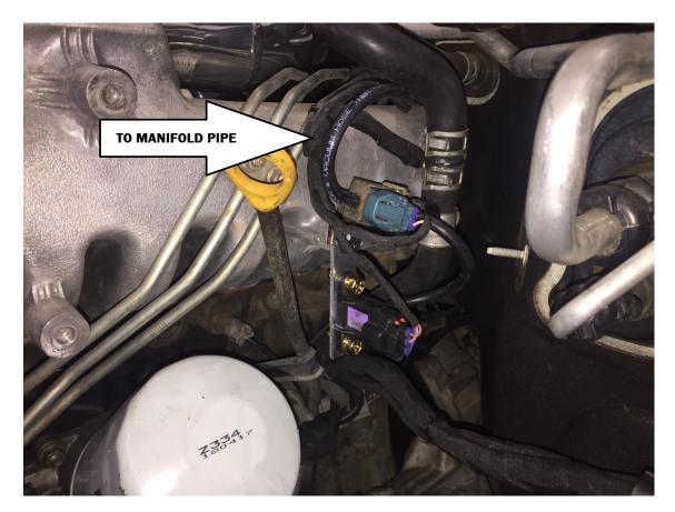
LOOP VAC HOSE FROM MAP SENSOR TO THE SOLENOID AND FROM THE SOLENOID TO THE BARB ON THE NEW CROSSOVER PIPE WHEN FITTED. THERE IS A SPARE PORT ON THE CROSSOVER PIPE FOR A BOOST GUAGE IF NEEDED.
