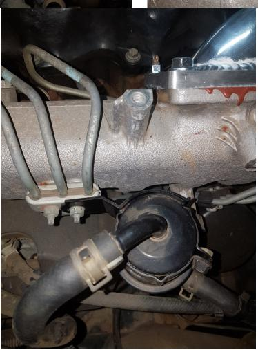
IF 100 SERIES FIT TEMP SENSOR TO MANIFOLD PIPE. IF 79 FIT TO TURBO PIPE. RUN VAC LINE FROM FITTING ON CROSSOVER PIPE TO SOLENOID AND MAP SENSOR AS SHOWN. RUN EXTENSION LOOM TO SHUT DOWN VALVE. INSTALL MANIFOLD USING SILICONE SEALANT. ASSEMBLE SILICONES AND PIPES AS SHOWN BELOW.
