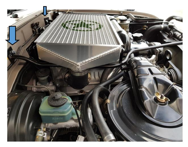
ASSAMBLE THE TWO FRAME RAILS TO THE INTERCOOLER USING THE 4X M8X16 BOLTS SUPPLIED. LIGHTLY TIGHTEN MOUNTING BOLTS IN THE BOTTOM OF THE SLOTS ON THE FRAME (END CLOSEST TO FRAME RAIL).
