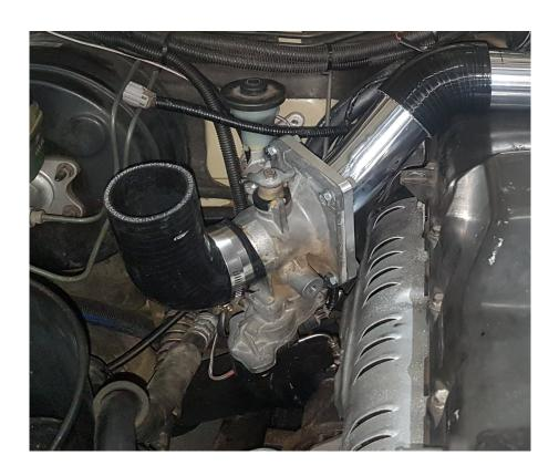
NOTE 100 SERIES ELECTRIC SHUT OFF VALVE SHOWN.
