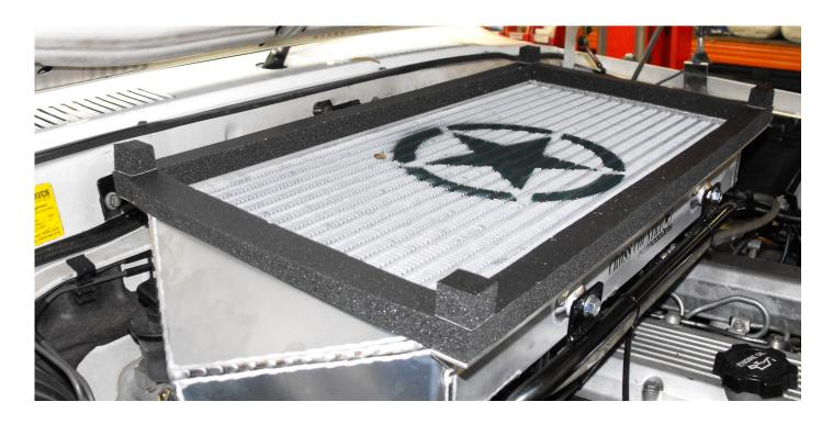
REMOVE BONNET AND SET ON TRESSLES. MARK THE FOUR FOAM SQAURES BEING SURE TO MARK ON THE INSIDE EDG OF THE SQUARES. REMOVE SQUARES AND DRILL THE TWO FRONT HOLES <u>ONLY</u> WITH A PILOT DRILL (3MM). CUT UNDER BONNET WEBBING OUT TO ALLOW APPROX 30-50MM CLEARANCE AROUND THE INTERCOOLER. THIS VARIES BETWEEN MODELS.
