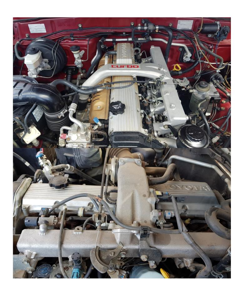
CARS FITTED WITH AN EGR, BLOCK VACUUM LINE RUNNING TO THE EGR DIAPHRAGM.
