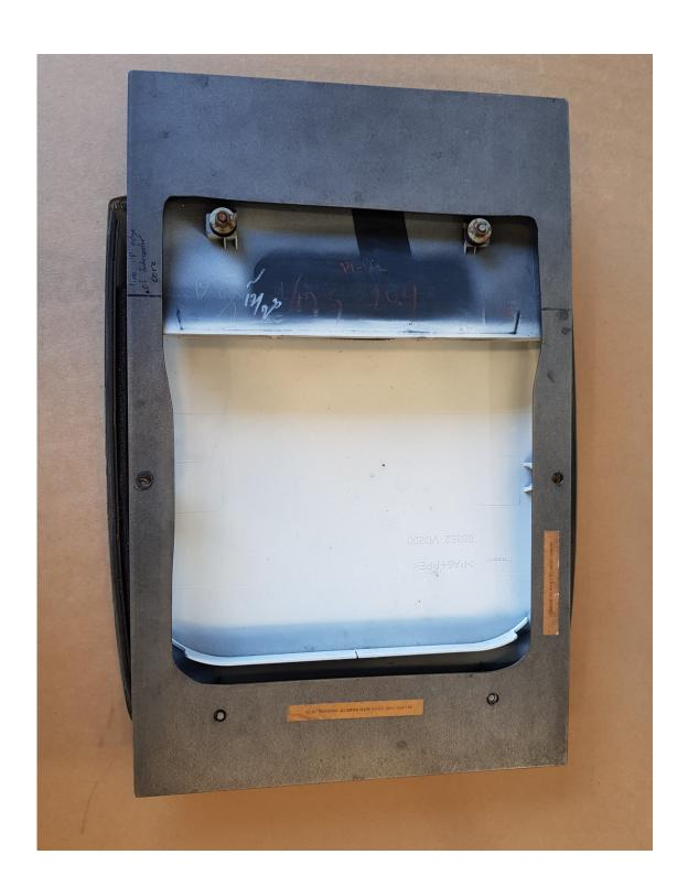
USING A GRINDER CUT OUT THE HOLE FOR THE INTERCOOLER USING MULTIPLE SHALLOW CUTS TO HELP PREVENT THE PAINT FROM BLISTERING. DRILL OUT MOUNTING HOLES.
