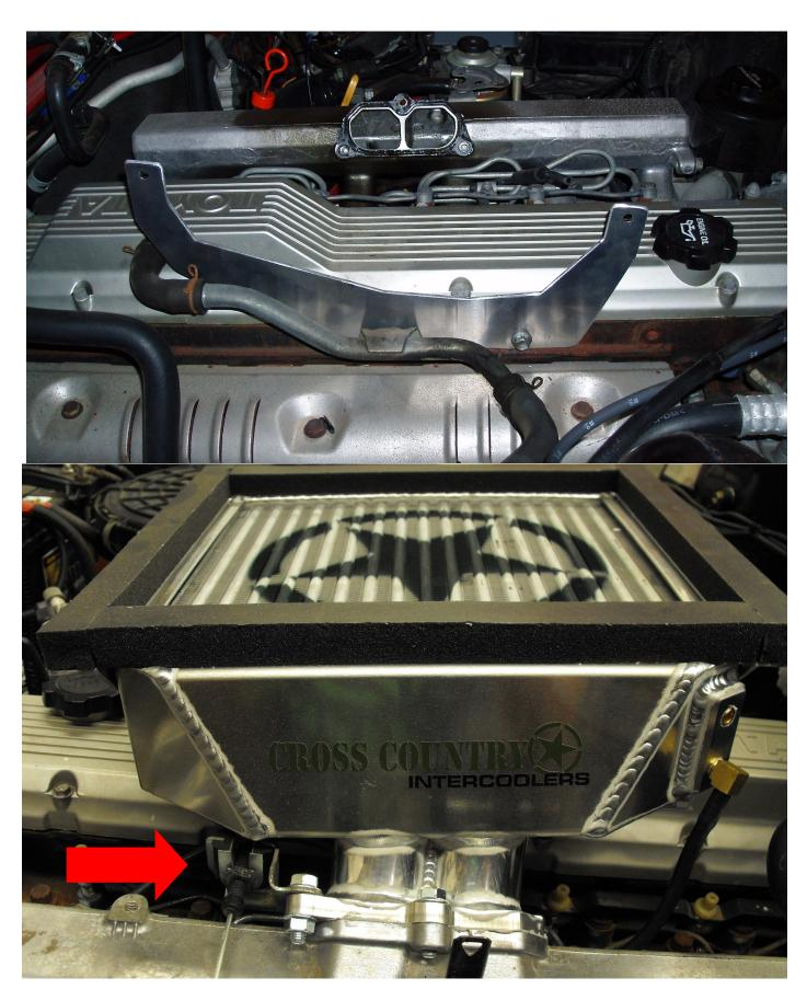
WITH INTERCOOLER FITTED TRIM AND INSTALL THE 2 45 DEGREE SILICONES TO THE TURBO SIDE OF THE INTERCOOLER. (NOTE OLD PICTURE SHOWN).
