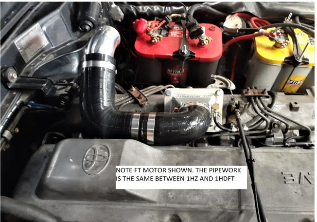
IF THE CAR IS EQUPPIED WITH A BOOST COMPENSATED FUEL PUMP USE THE SUPPLIED VACUUM HOSE TO RUN FROM THE FITTING ON THE INLET ADAPTOR TO THE BOOST COMPENSATOR. BLOCK OF NOT BEING USED.
