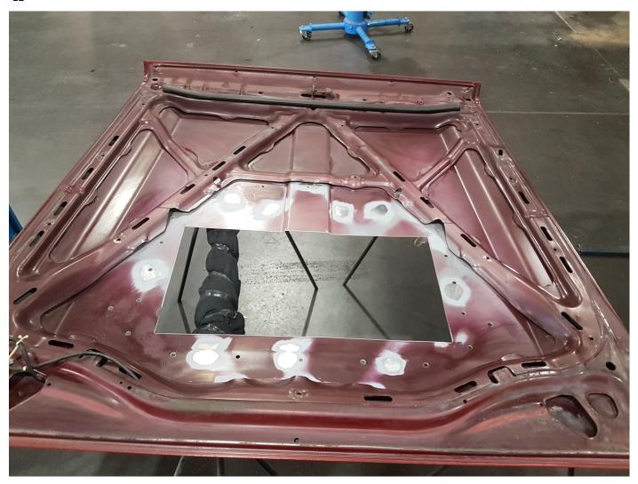
CUT WEBBING OUT AS SHOWN. THE WASHER JETS WILL NEED TO MOVED OUTWARDS TO CLEAR THE SCOOP. WHEN RE INSTALLING USE THE SUPPLIED CLEAR WASHER HOSE TO RECONNECT.
