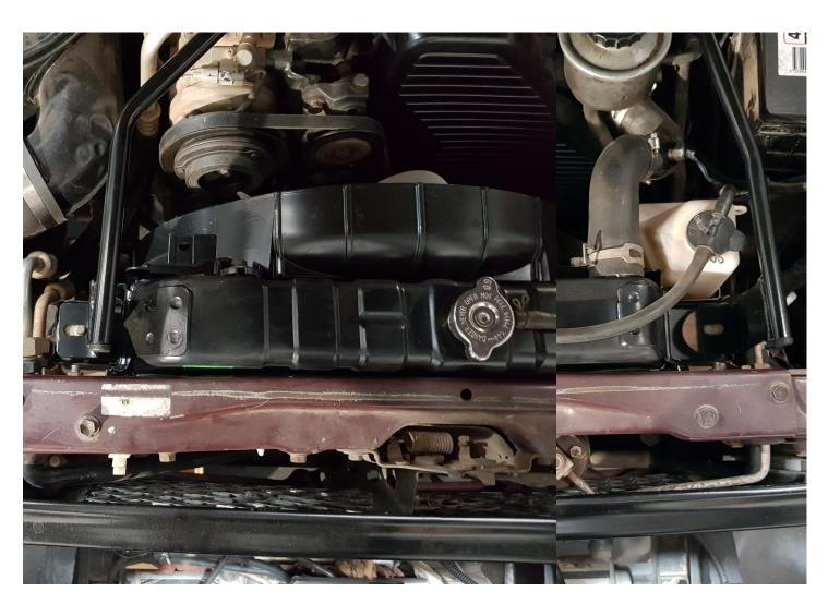
WITH THE INTERCOOLER FITTED TRIM AND FIT THE SILICONE TO THE REAR OF THE INTERCOOLER GIVING CLEARENE TO THE HEATER TAP AND TIGHTEN.
