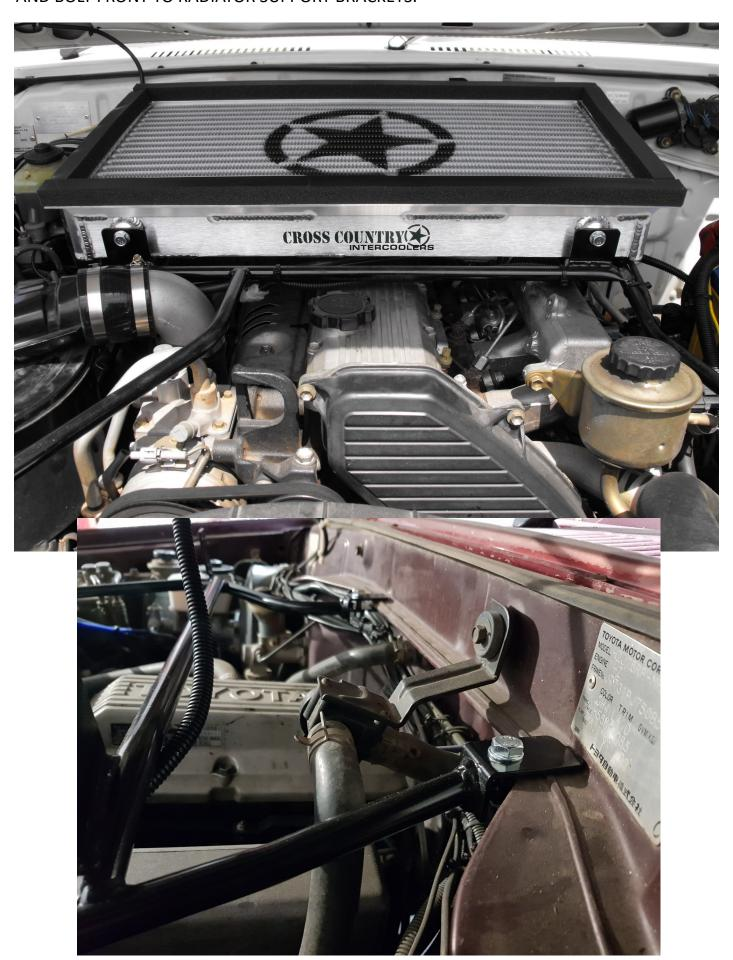
USE ADJUSTMENT IN THE FRONT FRAME TAGS TO GIVE ADEQUATE PURCHASE ON THE FIREWALL LIP AT THE REAR OF THE FRAME. AND BOLT DOWN USING M8 PANEL WASHER AND FACTORY NUTS. TIGHTEN THE REAR INTERCOOLER FRAME BOLTS SO THE FRAME CLAMPS THE LIP ON THE FIREWALL AS SHOWN
