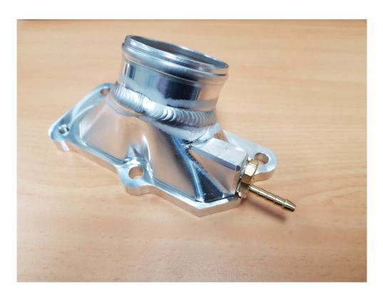
CHECK FOR ADEQUATE CLEARENCE TO THE THROTTLE CABLE BRACKET WHEN THE INTEROOLER IS INSTALLED.
