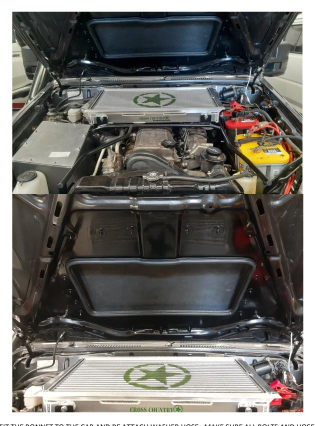
REFIT THE BONNET TO THE CAR AND RE ATTACH WASHER HOSE. MAKE SURE ALL BOLTS AND HOSE CLAMPS ARE TIGHT. CHECK FAN OPERATION AND TEST DRIVE VEHICLE AND CHECK FOR ANY LEAKS.
