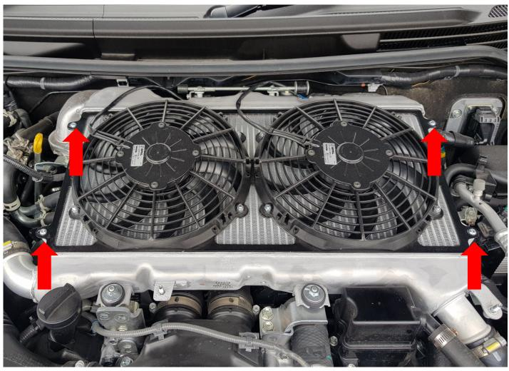
RUN THE FAN WIRES TO THE REAR OF THE INTERCOOLER AND REINSTALL FACTORY COVER.
