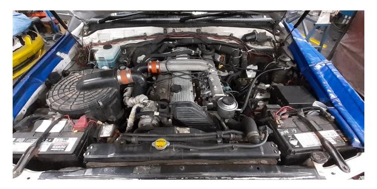
START WITH THE REMOVAL OF THE UNDERBONNET SOUND DEADENING KEEPING ALL THE CLIPS. REMOVE THE CROSSOVER PIPE AND PIPEWORK TO THE TURBO REMOVE CROSSOVER PIPE SUPPORT BRACKET. IF FITTED WITH AN EGR REMOVE EGR PIPE AND INSTALL EGR BLANK PLATE SUPPLIED.
