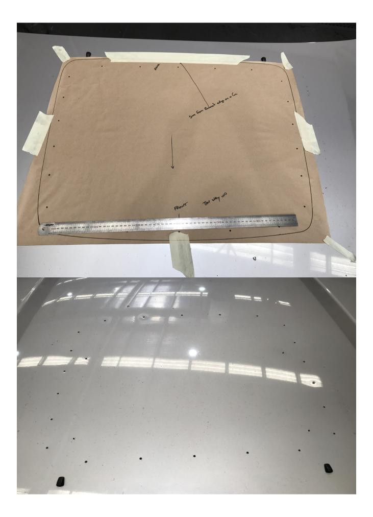
ONCE ALL SCOOP MOUNTING HOLES ARE DRILLED CUT OUT THE HOLE FOR THE INTERCOOLER AND PAINT ALL SURFACES.
