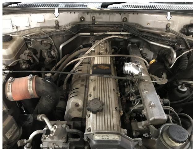
SOME AIRBOX TO TURBO PIPES WILL HAVE TO BE MODIFIED AS THE BREATHER FITTING MAY FOUL ON THE INTERCOOLER. FOR EXAMPLE THE BELOW DTS PIPE HAS BEEN MODIFIED TO MOVE THE BREATHER FITTING DOWN. THE AIRBOX LID MAY NEED TO BE ROTATED SLIGHTLY TO HELP CLEAR THE INTERCOOLER.
