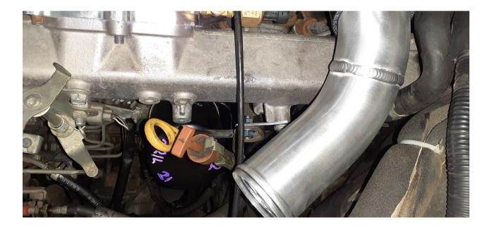
REMOVE BOLTS SHOWN ON FIREWALL. WHEN FITTING THE INTERCOOLER THE FRAME TAGS WILL GO BE-TWEEN THE FIREWALL AND THE BRACKETS HOLDING THE BRAKE LINES.
