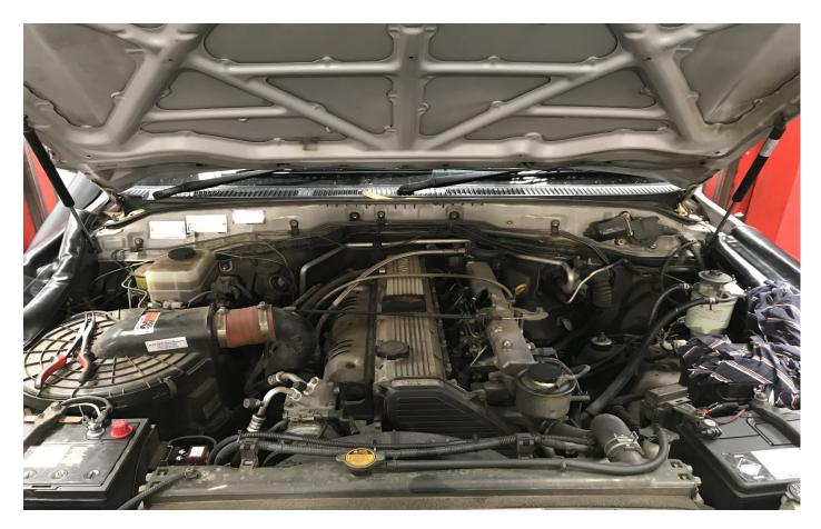
CARS FITTED WITH AN EGR, BLOCK VACUUM LINE RUNNING TO THE EGR DIAPHRAGM. LEAVE ALL OTHER SENSORS ATTACHED, MOVE THE BLACK SENSOR AND BLUE SOLENOID ON THE CROSSOVER PIPE WITH SUPPLIED BRACKET ONTO THE SIDE OF THE INTAKE MANIFOLD.
