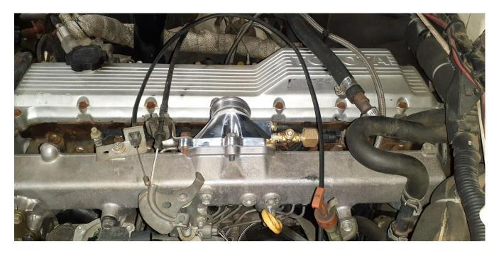
IF THE VEHICLE IS FITTED WITH AN ALTITUDE OR BOOST COMPENASTOR ON THE FUEL PUMP, RUN THE SUPPLIED VAC HOSE FROM THE FITTING ON THE INLET ADAPTOR TO THE TOP OF THE FUEL PUMP. ON A STOCK ALTITUDE COMPENSATED PUMP THE VACUUM LINE ON THE REAR OF THE PUMP WILL NEED TO BE VENTED TO THE ATMOSPHERE. IF YOU HAVE ANY QUESTIONS PLEASE CALL CROSS COUNTRY 4X4 ON 08 8357 5993
