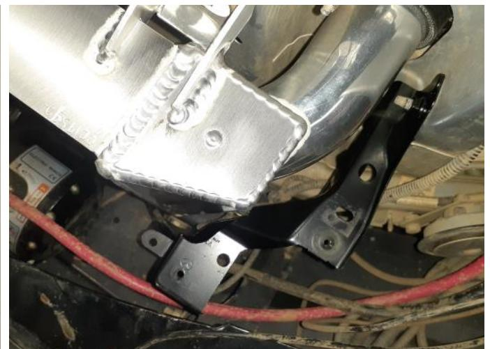
Remove the headlight supports and trim like shown on both sides allowing clearance for the intercooler.
